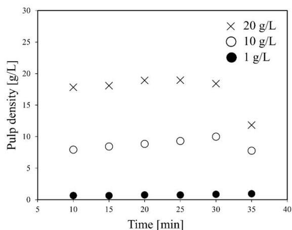
**Fig. 3** Effect of time on pulp density of recovered solution using flow line B. (LiCoO<sub>2</sub>, 30 ml/min)
