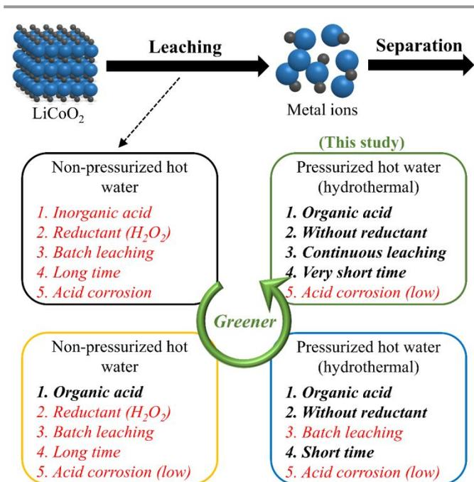
**Scheme 1** The green progress of acid leaching process for LiCo<sub>2</sub>. The words marked in red color are the problems to be resolved.
