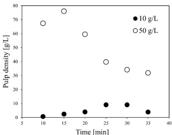
Fig. 1 Effect of time on pulp density of recovered solution using flow line A.
