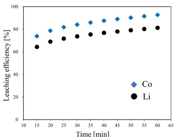
**Fig. 4** Effect of time on leaching efficiency of Li and Co during the continuous hydrothermal leaching of LiCoO<sub>2</sub> with H<sub>3</sub>Cit.
