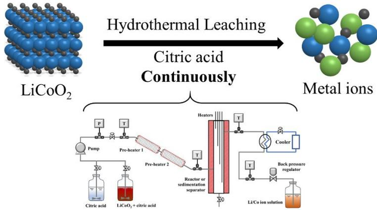
The continuous hydrothermal leaching of LiCoO<sub>2</sub> cathode materials with citric acid was firstly achieved using a customized flow system.
