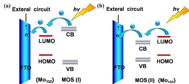
**Fig. 5** The scheme of the photo-induced electron transfer mechanism in the MOS electrodes. In 5a, MOS (I) represents a class of metal oxides, whose CB is higher than the LUMO of  $\{\text{Mo}_{132}\}$ .  $\{\text{Mo}_{132}\}$  clusters act as the electron acceptor. In 5b, MOS (II), the CB edge is lower than the LUMO of  $\{\text{Mo}_{132}\}$ .  $\{\text{Mo}_{132}\}$  clusters can be used as the electron donor.
