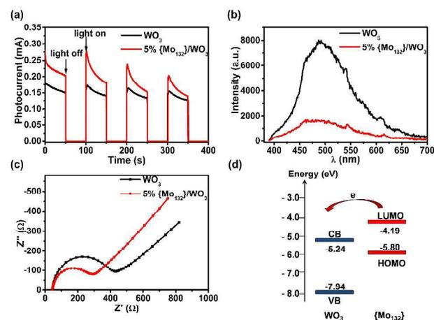
**Fig. 4** (a) Photocurrent responses of  $5\% \{\text{Mo}_{132}\}/\text{WO}_3$  (red line) and  $\text{WO}_3$  (black line). (b) Nyquist plots of  $5\% \{\text{Mo}_{132}\}/\text{WO}_3$  (red line) and  $\text{WO}_3$  (black line). (c) The emission spectra of  $5\% \{\text{Mo}_{132}\}/\text{WO}_3$  (red line) and  $\text{WO}_3$  (black line). (d) Energy levels of  $\text{WO}_3$  and  $\{\text{Mo}_{132}\}$ .
