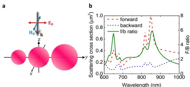
**Figure 9.** (a) Schematic image of the configuration used in calculation. (b) Scattering spectra of the trimer. Scattering cross section to the forward and backward direction and F/B ratio of the trimer using silicon spheres of 165 nm, 225 nm and 310 nm diameter.
