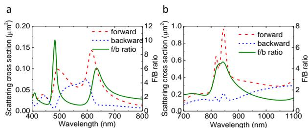
**Figure 6.** Scattering properties shifted to the boundaries of the visible regime. Spectra of scattering cross sections to the forward and backward directions and F/B ratio of the dimer using silicon spheres of 110 nm and 150 nm diameter (a) and the dimer using silicon spheres of 225 nm and 310 nm diameter (b).
