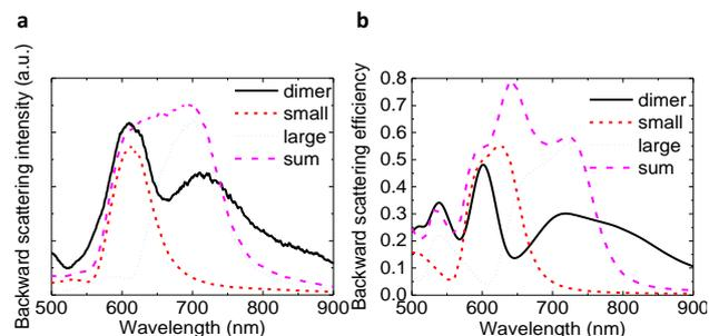
**Figure 8** Comparison of experimental (a) and theoretical (b) scattering spectra to the backward direction of the single disks, the numerical sum of these two disks and the dimer configuration.
