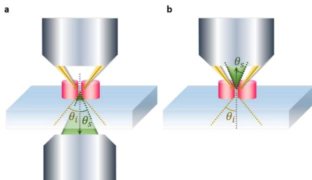
**Figure 1.** Schematic images of the optical measurement setup. Detailed illustration of the darkfield single nanoantenna measurement setups for the forward scattering (a) and backward scattering (b).
