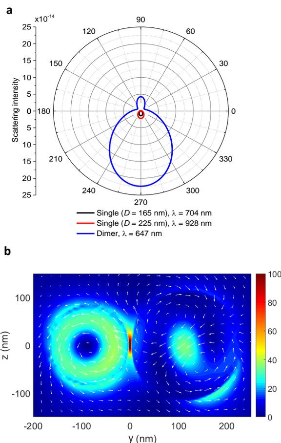
**Figure 3.** (a) Scattering pattern in far field from the single spheres and dimer configuration projected in x-z plane. (b) Electric field intensity and coupling between the resonances. Cross section of electric field intensity inside and near the dimer configuration at 647 nm illumination in the y-z plane. White arrows in the figure show the real part of electric field vectors at each calculation cell.
