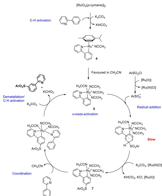
Scheme 5 Proposed catalytic cycle
