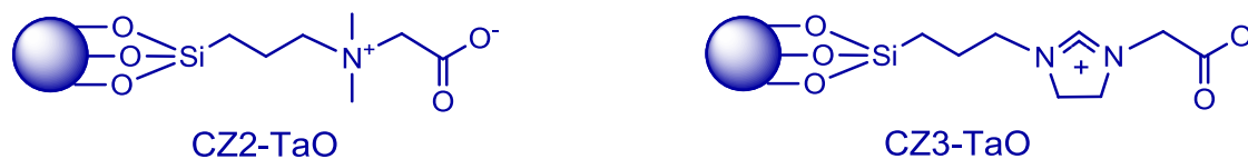
Figure 1 Graphical representations of CZ2-TaO and CZ3-TaO nanoparticle contrast agents with TaO core and ligand shell
