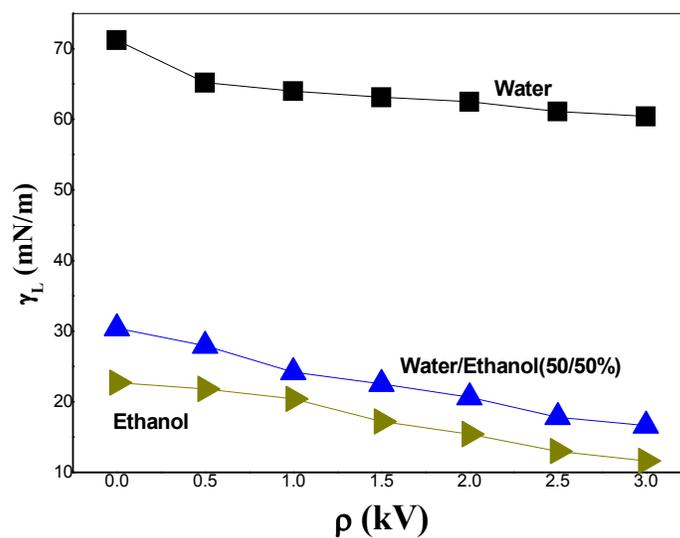
*Figure 5. Effect of applied voltages on the surface tension of water/ethanol mixtures.*
