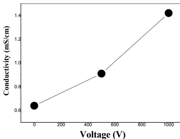
*Figure 5. Effect of applied voltages on the conductivity of BaF<sub>2</sub> nanocrystals prepared by electric-assisted phase separation and precipitation.*
