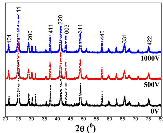
*Figure 3. XRD patterns of  $\text{BaF}_2$  nanocrystals prepared by electric-assisted phase separation and precipitation.*
