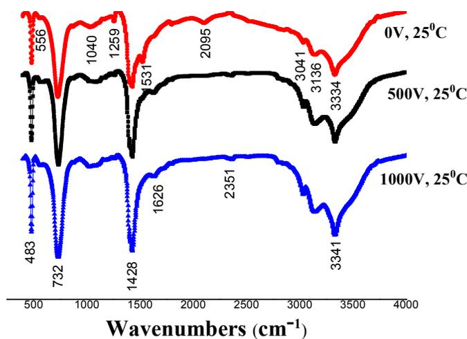
*Figure 4. FTIR spectra of  $\text{BaF}_2$  nanocrystals prepared by electric-assisted phase separation and precipitation method.*
