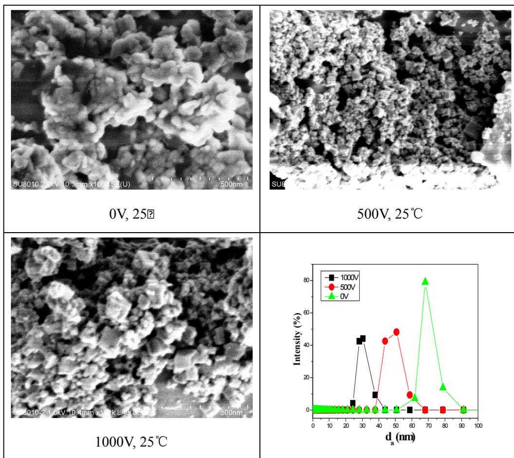
*Figure 2. FESEM images and particle size distribution of BaF<sub>2</sub> nanocrystallites formed by electric-assisted phase separation and precipitation in water/ethanol mixture.*
