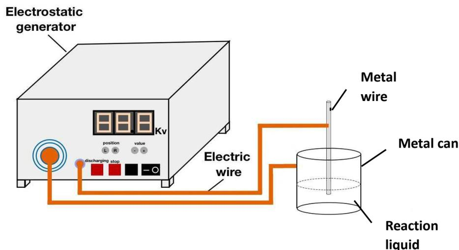
*Figure 1. Scheme on the application of the electric-assisted phase separation and precipitation method to form nanocrystals.*
