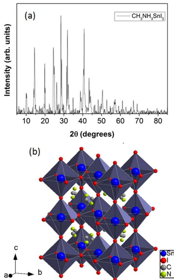
**Figure 1: X-ray Diffraction (XRD) and Crystal Structure.** (a) XRD pattern derived from a ground powder of  $\text{CH}_3\text{NH}_3\text{SnI}_3$ . (b) Simulated crystal structure of  $\text{CH}_3\text{NH}_3\text{SnI}_3$  obtained from the diffraction pattern given in (a) showing the tetragonal conformation of the perovskite lattice.
