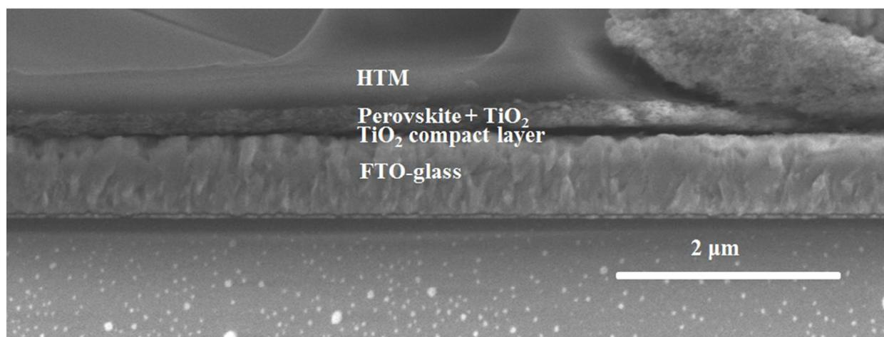
**Figure S3: Cross-Sectional Scanning Electron Microscope (SEM) Image.** Cross-sectional SEM image of a  $\text{TiO}_2$ -based  $\text{CH}_3\text{NH}_3\text{SnI}_3$  device.
