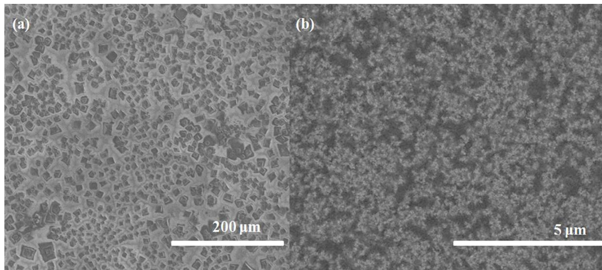
**Figure S4: Top-View Scanning Electron Microscope Images.** Top view SEM image of (a) A capping layer of disperse  $\text{CH}_3\text{NH}_3\text{SnI}_3$  crystal formed on an 80 nm thick film of  $\text{TiO}_2$ . (b)  $\text{CH}_3\text{NH}_3\text{SnI}_3$  coated on a 400 nm thick film of  $\text{TiO}_2$  such that all of the crystallites have formed within the pores of the  $\text{TiO}_2$  and no capping layer is present.
