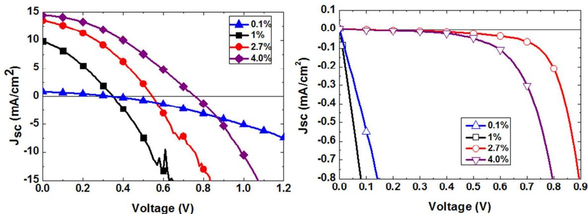
**Figure S5: Current-Voltage Characteristics of Various  $\text{CH}_3\text{NH}_3\text{SnI}_3$  Devices.** (a) Current-voltage (JV) characteristics of  $\text{CH}_3\text{NH}_3\text{SnI}_3$  devices of a spread power conversion efficiencies (PCE) under illumination. The PCEs of the devices are as follows: 0.1% (blue triangles), 1% (black squares), 2.7 % (red circles), 4.0% (purple diamonds). (b) Corresponding dark JV characteristics for the devices shown in (a), represented by hollow symbols.
