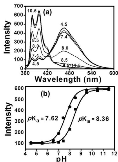
Fig. 2 (a) Fluorescence response of **1** (10 μM) in the absence of carbohydrate at different pHs and (b) the emission intensity at 378 nm as a function of pH in the presence (●) and absence (■) of glucose (0.05M) in a 50 mM phosphate buffer solution containing 1% DMSO.
