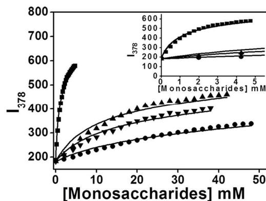
Fig. 3 Emission intensity of **1** (10 μM) upon addition of D-glucose (●), D-galactose (▲), D-mannose (▼) and D-fructose (■) in 50 mM phosphate buffer solution containing 1% DMSO at pH 7.4.
