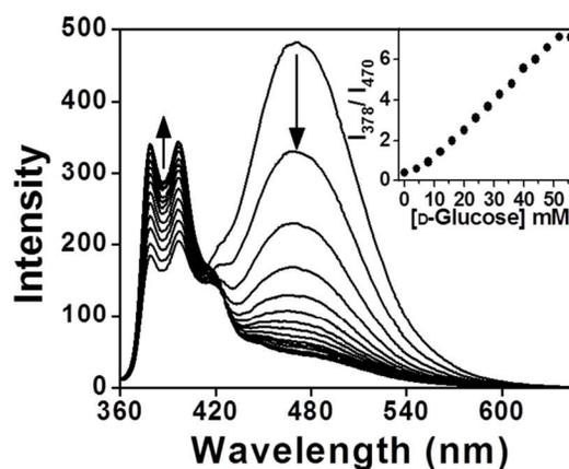
70 **Fig. 1** Fluorescence emission spectra of **1** (10 μM) upon addition of D-glucose (0 – 0.056 M) ( $\lambda_{\text{ex}} = 342$  nm) in 50 mM phosphate buffer solution containing 1% DMSO at pH 7.4.
