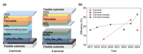
Fig. 16 (a) Schematic illustration of 2T and 4T configurations of CIGS-perovskite tandem solar cells. (b) Diagram showing recent improvements in the efficiency of 2T and 4T flexible CIGS-perovskite tandem solar cells.
