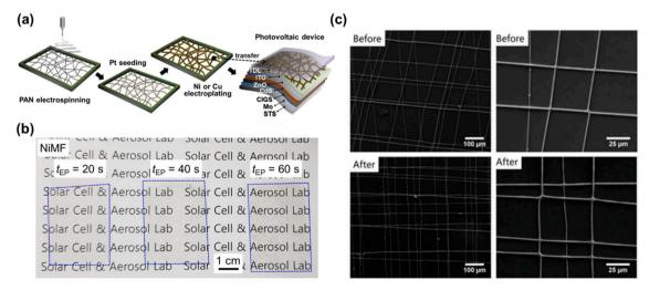
Fig. 2 (a) Schematic illustration showing the fabrication and transfer of metal microfibers onto flexible CIGS solar cells. (b) Ni microfibers subjected to electroplating durations ( $t_{EP}$ ) of 20, 40, and 60 s. ((a) and (b) Reproduced from ref. 73 with permission from Elsevier, Copyright 2024) (c) scanning electron microscopy (SEM) images of Ag mesh grids on PET substrates before and after flash lamp annealing. (Reproduced from ref. 74 with permission from Taylor & Francis, Copyright 2018).
