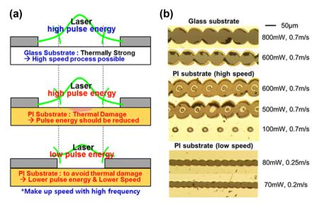
Fig. 6 (a) Schematic illustrations of P1 laser scribing mechanisms for SLG and P1 substrate samples. (b) Optical images of P1-scribed samples for ITO and Pl substrates. Both samples were coated with a 1-µm-thick Mo layer. (Reproduced from ref. 106 with permission from Springer Nature, Copyright 2016).
