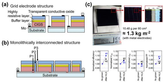
Fig. 5 (a) Schematic illustrations of grid electrode-connected and monolithically interconnected module structures. (b) Photograph of CIGS solar minimodule. (c) Module performance with and without heat-light soaking. (Reproduced from ref. 8 with permission from Springer Nature, Copyright 2022).
