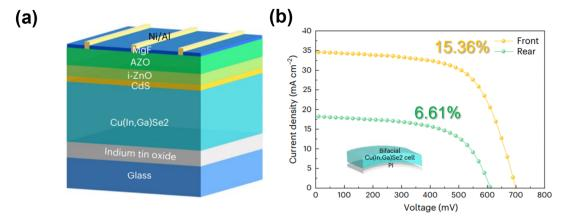
Fig. 14 (a) Device structure of a bifacial CIGS solar cell fabricated on a glass substrate. (b) J-V curves of flexible bifacial CIGS device under front and rear illumination, with a simplified scheme of the device architecture. (Reproduced and adapted from ref. 142 with permission from Springer Nature, Copyright 2022).
