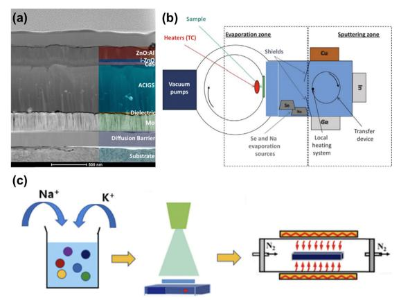
Fig. 3 (a) Structure of flexible solar cell with an Aq-alloyed CIGS absorber layer. (Reproduced from ref. 76 with permission from Springer Nature, Copyright 2023) (b) schematic illustration of hybrid sputtering-evaporation method. (Reproduced from ref. 78 with permission from Elsevier, Copyright 2018) (c) schematic illustration of aqueous spray deposition and selenization processes. (Reproduced from ref. 81 with permission from Elsevier, Copyright 2022)
