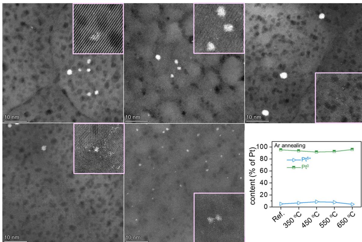
Fig. 7 Impact of thermal annealing in argon on the light-induced agglomeration behavior of Pt species on flat TiO<sub>2</sub> films (top left to bottom right: as-deposited; 350 °C, 1 h; 450 °C, 1 h; 550 °C, 1 h; 650 °C, 1 h; Pt<sup>δ+</sup> to Pt<sup>0</sup> ratio as determined by XPS).
