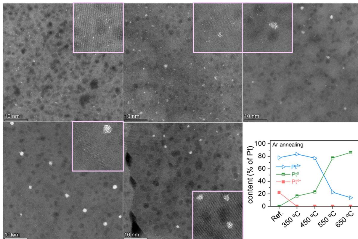
Fig. 3 Impact of thermal annealing in an argon atmosphere on the Pt dispersion and agglomeration on flat  $\text{TiO}_2$  films (top left to bottom right: as-deposited; 350 °C, 1 h; 450 °C, 1 h; 550 °C, 1 h; 650 °C, 1 h;  $\text{Pt}^{6+}$  to  $\text{Pt}^0$  ratio as determined by XPS).
