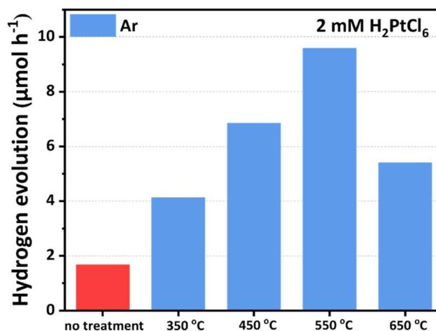
Fig. 1 Impact of thermal annealing in an Ar atmosphere on the photocatalytic activity of Pt dispersed on flat TiO<sub>2</sub> films.
