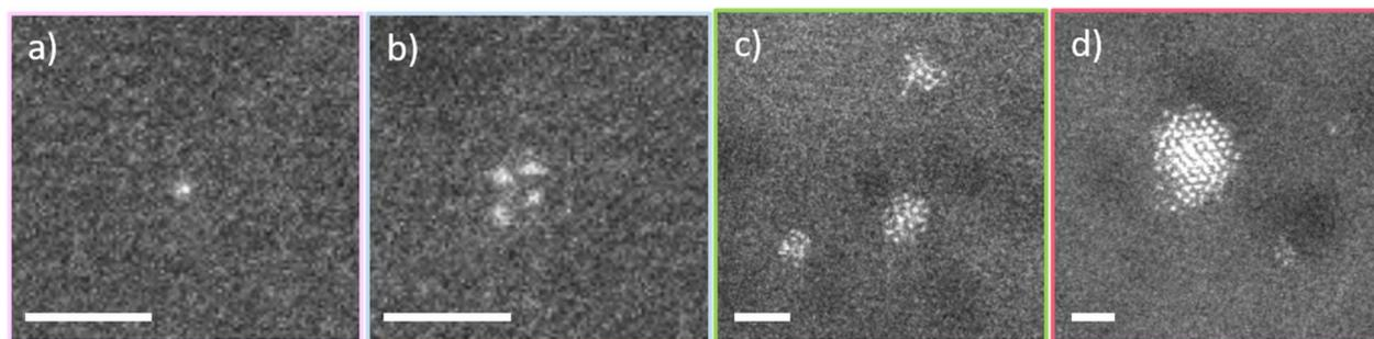
Fig. 2 Different types of Pt species typically co-existing on the  $\text{TiO}_2$  support: (a) SA, (b) a few-atom raft, (c) rafts exhibiting a disordered structure, and (d) a NP showing lattice fringes (the scale bar corresponds to 1 nm).
