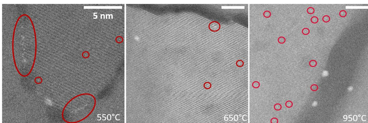
Fig. 5 High-magnification *in situ* HAADF-STEM observations of Pt SAs (highlighted) at different temperatures (following the same procedure as in Fig. 4). The scale bar in all images corresponds to 5 nm.
