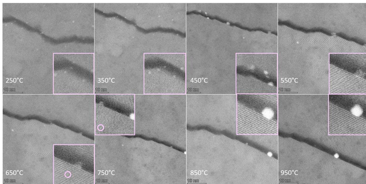
Fig. 4 Identical-location *in situ* HAADF-STEM images of the Pt SA decorated TiO<sub>2</sub> layer (using 0.05 mM H<sub>2</sub>PtCl<sub>6</sub>) heated in an Ar atmosphere (700 mbar) to different temperatures (250–950 °C). Pt species can be identified as bright spots on the TiO<sub>2</sub> surface (based on the significant difference in atomic number between Pt (78) and Ti (22), and the related scattering strength in HAADF-STEM imaging).
