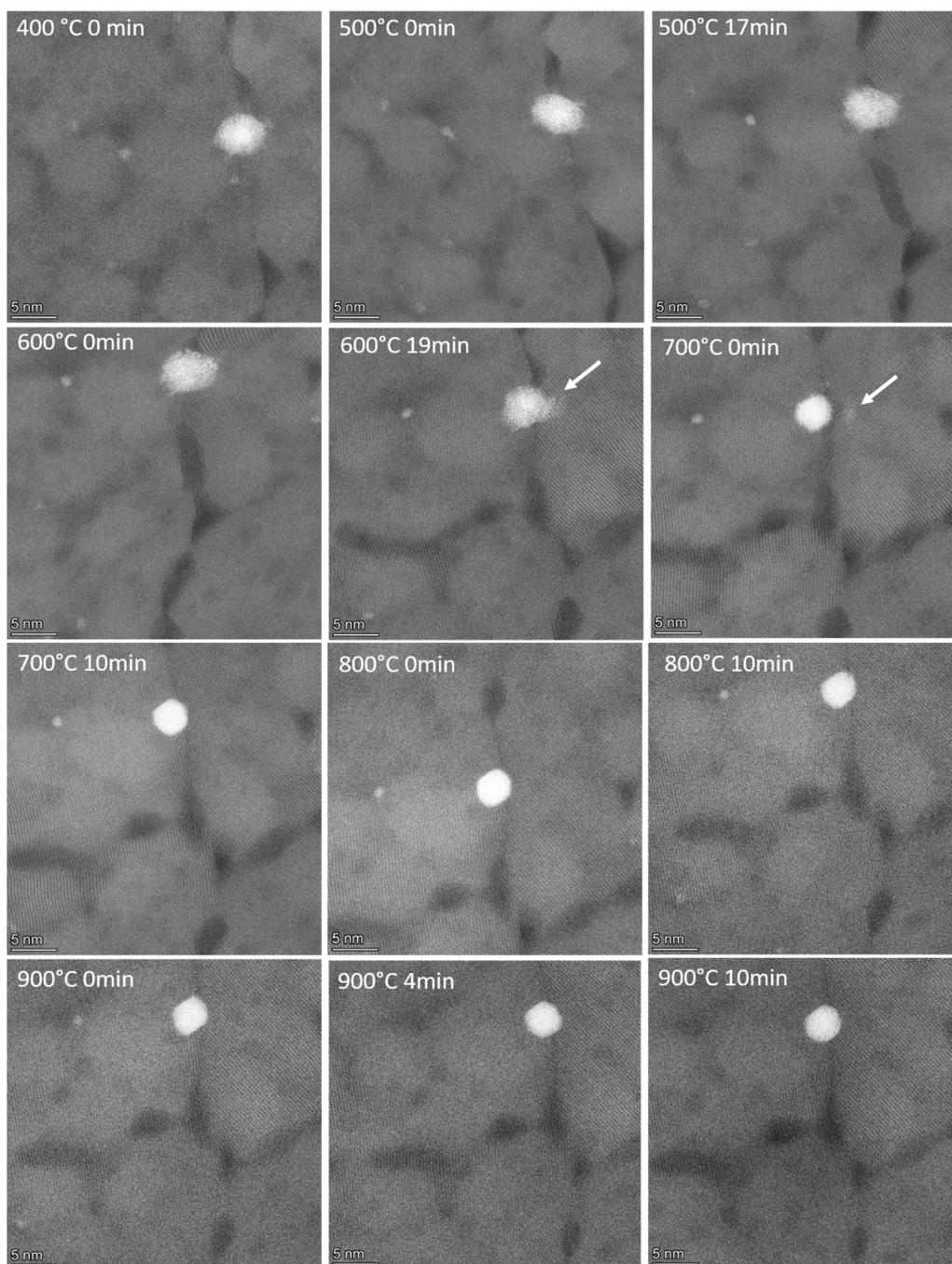
Fig. 6 High-magnification identical-location *in situ* HAADF-STEM imaging series showing the evolution of a Pt nucleus and its surroundings at 400–900 °C. The white arrow indicates the detachment of a Pt cluster from a larger particle.
