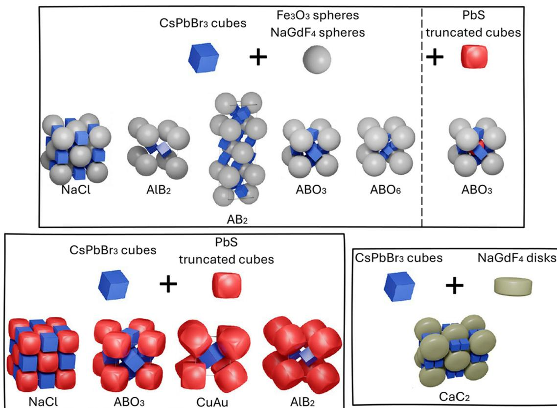
Fig. 20 Diversity of binary and ternary superstructures obtained from 5.3 and 8.6 nm cubic  $\text{CsPbBr}_3$  nanoparticles combined with 11.2–25.1 nm spherical  $\text{Fe}_3\text{O}_4$  and  $\text{NaGdF}_4$  nanoparticles, 10.7–11.7 nm truncated cuboid PbS nanoparticles, and  $\text{NaGdF}_4$  disks (31.5 nm in diameter and 18.5 nm thick). Adapted with permission from ref. 240. Copyright 2022 American Chemical Society.
