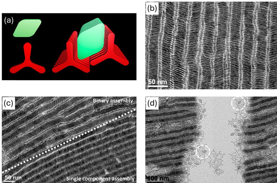
Fig. 25 (a) Schematic illustration of rhombic, tripodal nanoplates, and binary assembly. TEM images of (b) a binary co-assembly of tripodal and rhombic nanoplates formed *via* complementary-shape interaction, (c) a binary superstructure domain bordering a single-component superstructure domain of rhombic nanoplates, and (d) a fractured binary superstructure consisting of co-assembled tripodal and rhombic nanoplates. Adapted with permission from ref. 237. Copyright 2013 American Chemical Society.
