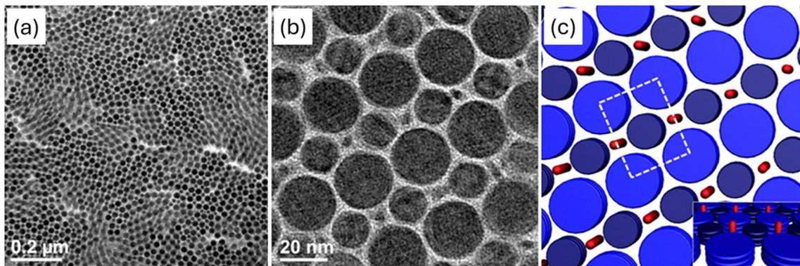
Fig. 28 (a) and (b) TEM images and (c) the structural model of an LMS-type superstructure co-assembled from small and large  $\text{LaF}_3$  nanodisks and  $\text{CdSe/CdS}$  nanorods. Adapted with permission from ref. 235. Copyright 2015 American Chemical Society.
