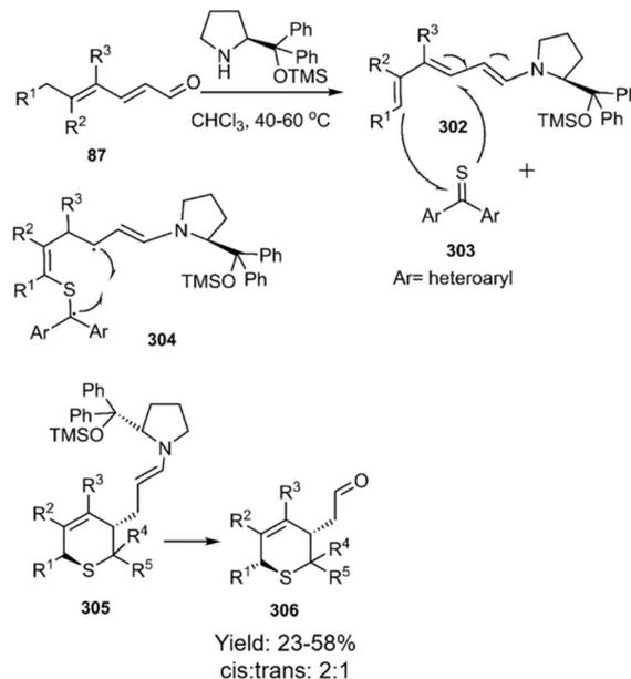
Scheme 87 Mechanism of enantioselective synthesis of thiopyrans **306**.
