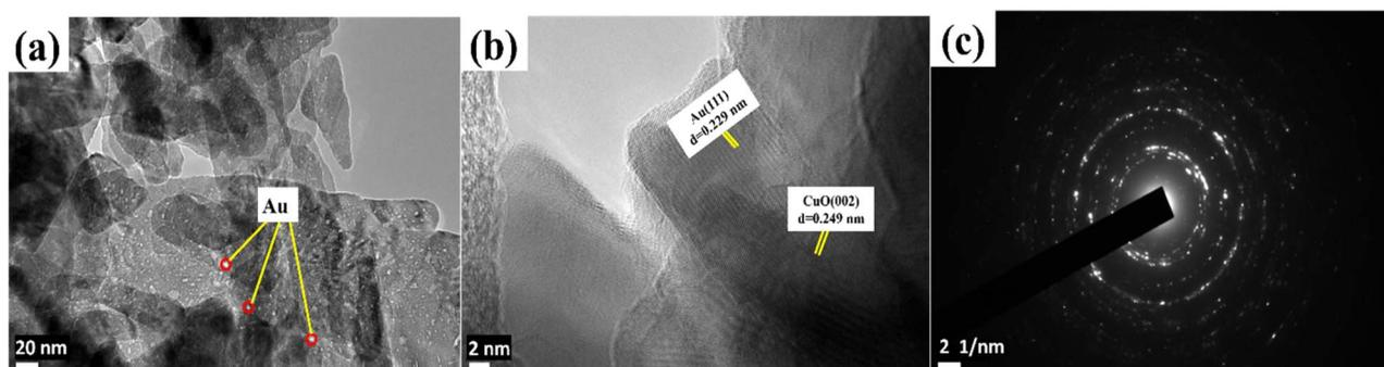
Fig. 4 TEM image of (a) the Au@rGO/CuO nanocomposite, (b) HR-TEM image of the Au@rGO/CuO nanocomposite, and (c) the SAED pattern of the Au@rGO/CuO nanocomposite.
