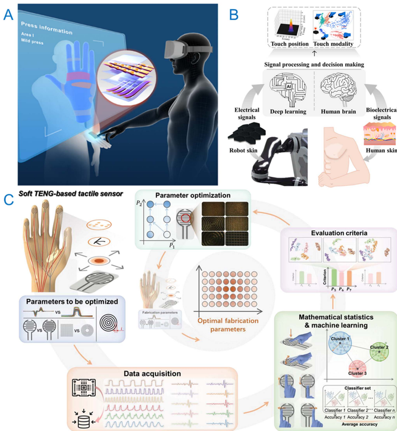
Fig. 1 (A) Next-generation intelligent sensing integrated with AI signal processing. 22 (B) The similarity between human brain learning and deep learning. 23 (C) Schematic diagram of sensor design assisted by machine learning through parameter optimization. 9
