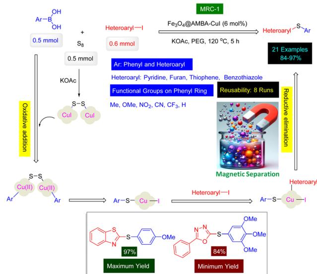
Scheme 1 Fe<sub>3</sub>O<sub>4</sub>@AMBA-CuI (MRC-1) catalyzed synthesis of heteroaryl-aryl and di-heteroaryl sulfides from S<sub>8</sub>.
