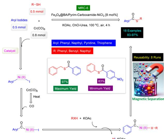
Scheme 6 Fe<sub>3</sub>O<sub>4</sub>@BA/Pyrim-carboxamide-NiCl<sub>2</sub> (MRC-6) catalyzed preparation of thioesters from thiols.
