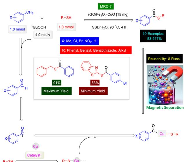
Scheme 7 rGO/Fe<sub>3</sub>O<sub>4</sub>-CuO (MRC-7) catalyzed preparation of thioesters from thiols.
