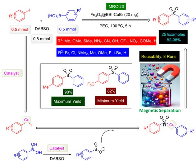
Scheme 23 Fe<sub>3</sub>O<sub>4</sub>@BBI-CuBr nanomaterial (MRC-23) catalyzed preparation of diaryl sulfone derivatives from DABSO.
