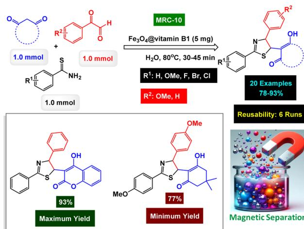
Scheme 10 Fe<sub>3</sub>O<sub>4</sub>@vitamin B1 nanomaterial (MRC-10) catalyzed preparation of trisubstituted 1,3-thiazole derivatives from thioamides.
