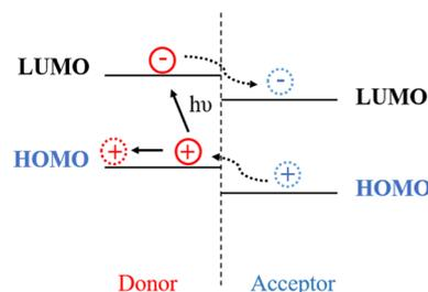
Fig. 1 Working principle of organic solar cells.
