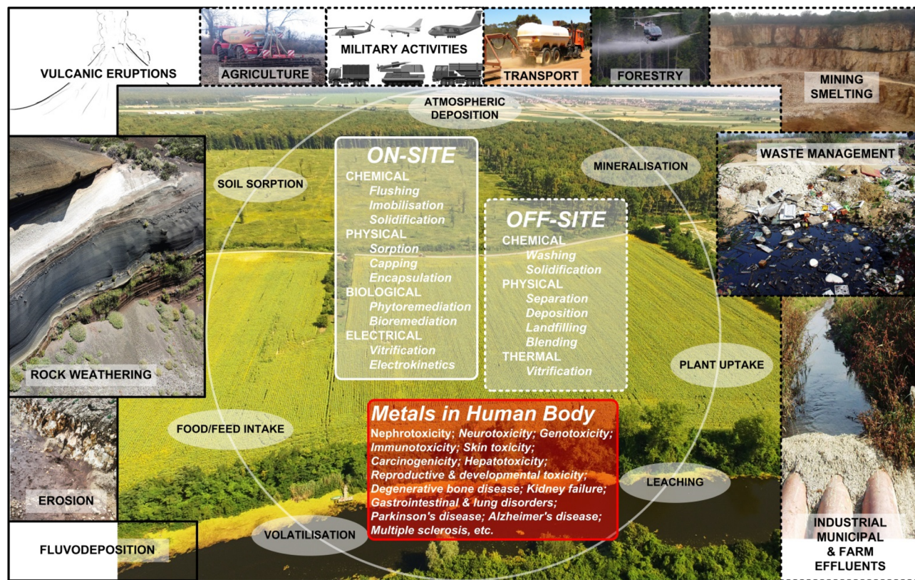
Fig. 1 Schematic representation of the most important natural (rectangles bordered by solid black lines) and anthropogenic (rectangles with dashed black lines) sources of metal contamination, with metal transfer pathways (ovals) in the environment as well as into the human food chain, and on-site and off-site approaches to remediate metal-contaminated soils.
