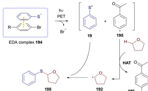
**Scheme 27** Akiyama's work on C(sp<sup>3</sup>)-S bond forming transformations through the activation of C(sp<sup>3</sup>)-H bonds.
