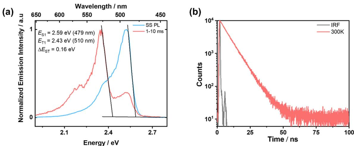
**Fig. 5** (a) Steady-state PL and phosphorescence spectra of **2,7-tBuCzNB** ( $\lambda_{\text{exc}} = 340$  nm). (b) Time-resolved PL decay of **2,7-tBuCzNB** in degassed toluene ( $\lambda_{\text{exc}} = 375$  nm).
