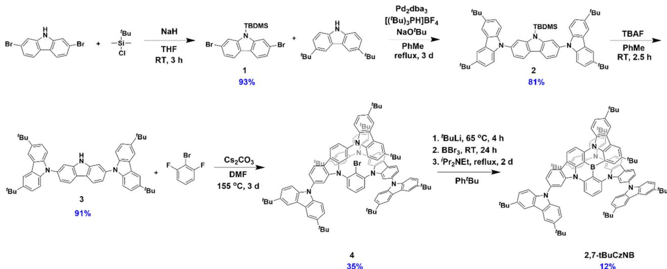
Fig. 2 Synthesis scheme of 2,7-tBuCzNB.
