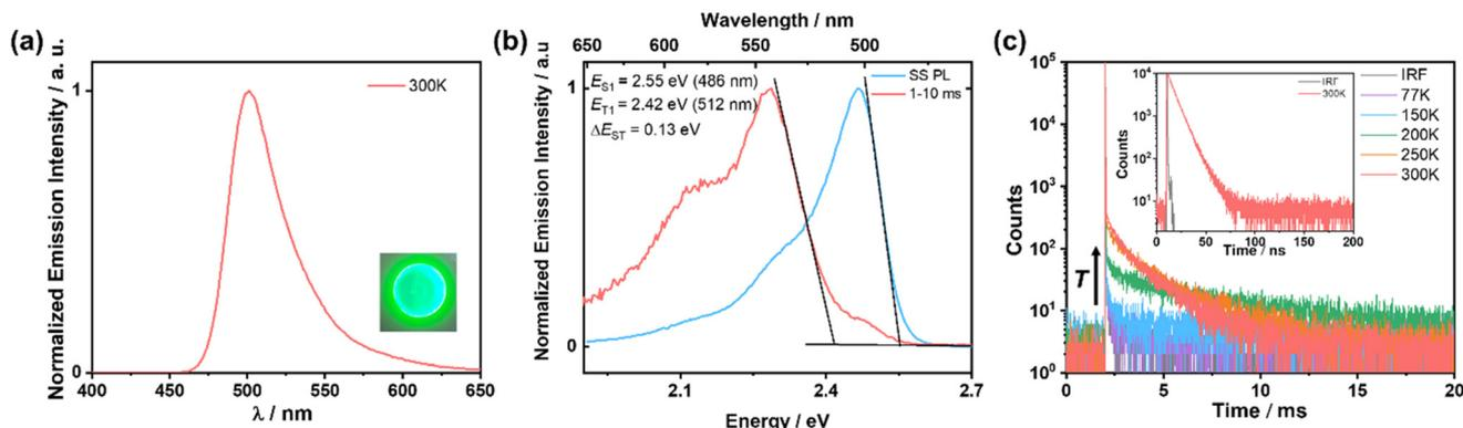
**Fig. 6** (a) Steady-state PL spectra in the 5 wt% doped film in mCP ( $\lambda_{\text{exc}} = 340$  nm). Inset: photo of the doped film excited at 365 nm. (b) Steady-state PL and phosphorescence spectra of the 5 wt% doped film of **2,7-tBuCzNB** in mCP measured in the film at 77 K ( $\lambda_{\text{exc}} = 340$  nm). (c) Variable temperature time-resolved PL decays of the 5 wt% doped film of **2,7-tBuCzNB** in mCP ( $\lambda_{\text{exc}} = 375$  nm).
