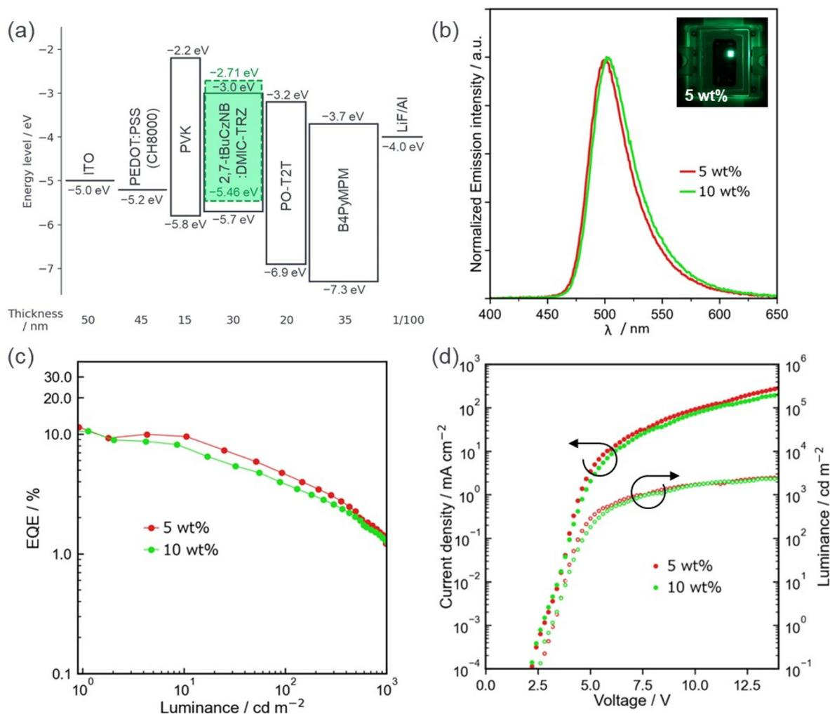
**Fig. 7** (a) Device structure, (b) electroluminescence spectra (inset: photograph of the 5 wt% device), (c) EQE–luminance curves, and (d) current density–voltage–luminance characteristics of SP-OLEDs using 5 or 10 wt% 2,7-*t*BuCzNB:DMIC-TRZ as the emitting layer.
