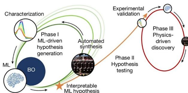
**Fig. 13** The closed-loop transfer (CLT) diagram. Phase I involves ML-driven reaction discovery and optimization. In phase II, ML-generated hypotheses are experimentally validated, leading to phase III, where physics-driven discovery generates new insights into molecular catalysis. Reprint with permission request from ref. 133, copyright 2024, Springer Nature.
