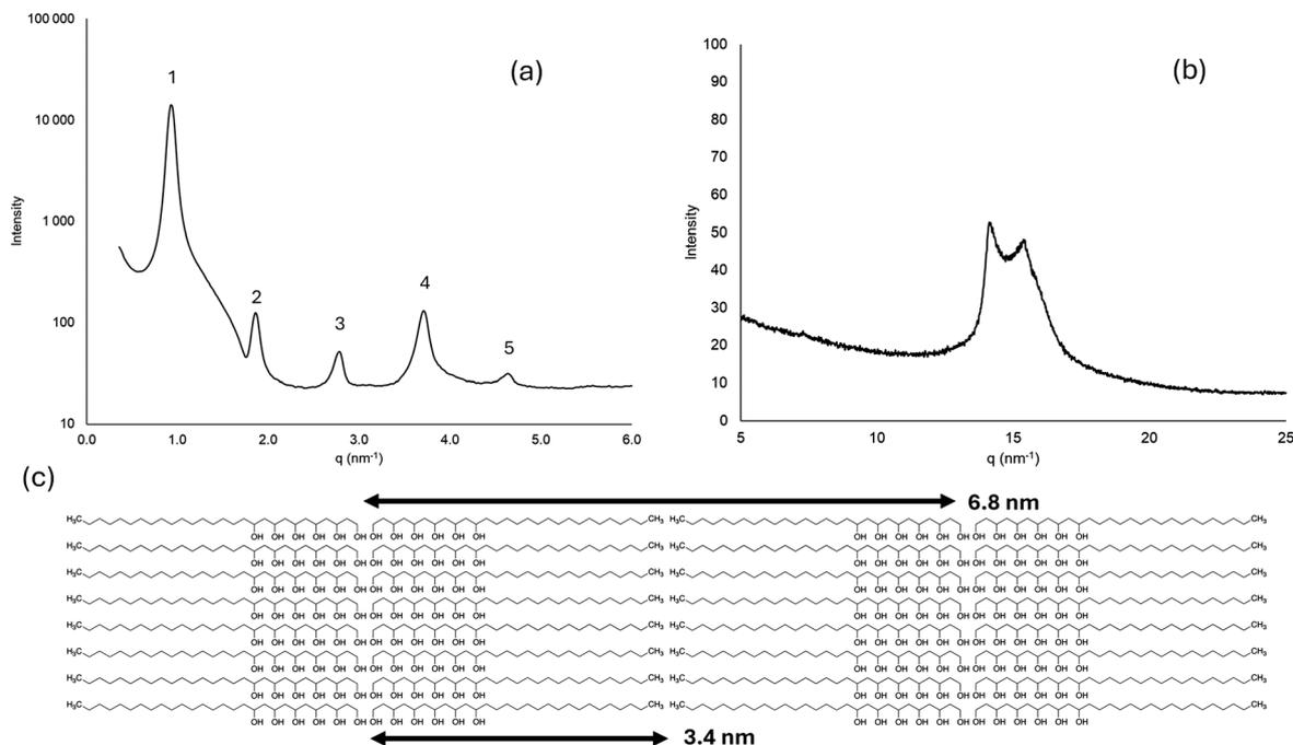
**Fig. 6** SAXS (a) and WAXS (b) patterns at room temperature of oligomers with  $n = 5$  VA units and the corresponding proposed structure (c) formed in the solid state (the dimensions shown are calculated using the C–C bond length, assuming a fully extended conformation).
