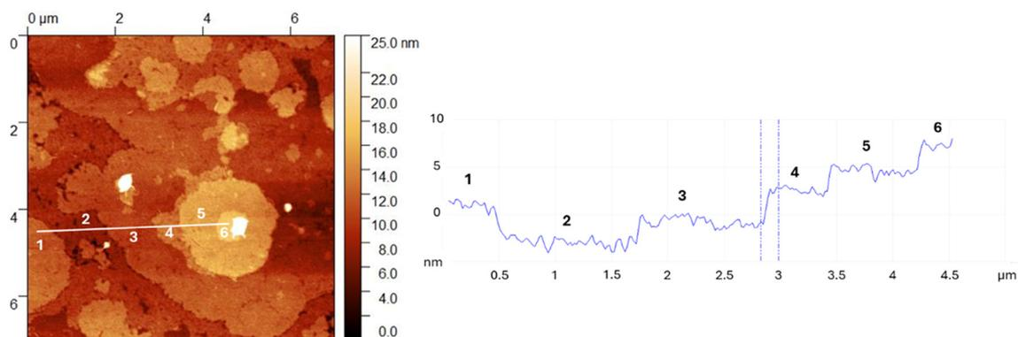
Fig. 7 AFM image ( $7 \times 7 \mu\text{m}$ ) (left) and the corresponding height line profile (right) showing flat terraces for oligomers with  $n = 5$  VA units, spin coated on a glass substrate and annealed above  $T_{\text{ODT}}$ .
