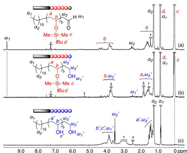
**Fig. 4** <sup>1</sup>H NMR spectra of the original oligomer ( $n = 5$ ) (a) and the oligomer obtained after reduction (b) and deprotection (c) (CDCl<sub>3</sub> at 55 °C for a and b, DMSO-*d*<sub>6</sub> at 100 °C for c). \*CHCl<sub>3</sub>, <sup>†</sup>water, <sup>‡</sup>CH<sub>2</sub>Cl<sub>2</sub>, <sup>§</sup>THF, and <sup>#</sup>DMSO.
