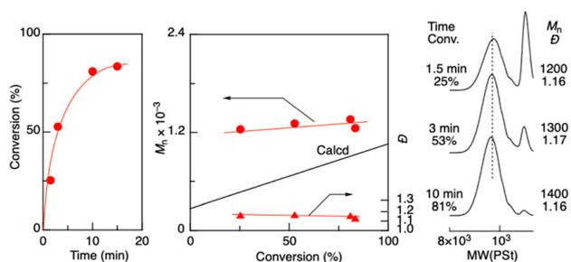
**Fig. 1** Aldol-GTP of TBSVE with octadecyl aldehyde as an initiator and  $\text{ZnBr}_2$  as a catalyst:  $[\text{TBSVE}]_0/[\text{octadecyl aldehyde}]_0/[\text{ZnBr}_2]_0 = 500/100/20$  mM in  $\text{CH}_2\text{Cl}_2$  at  $0^\circ\text{C}$ .
