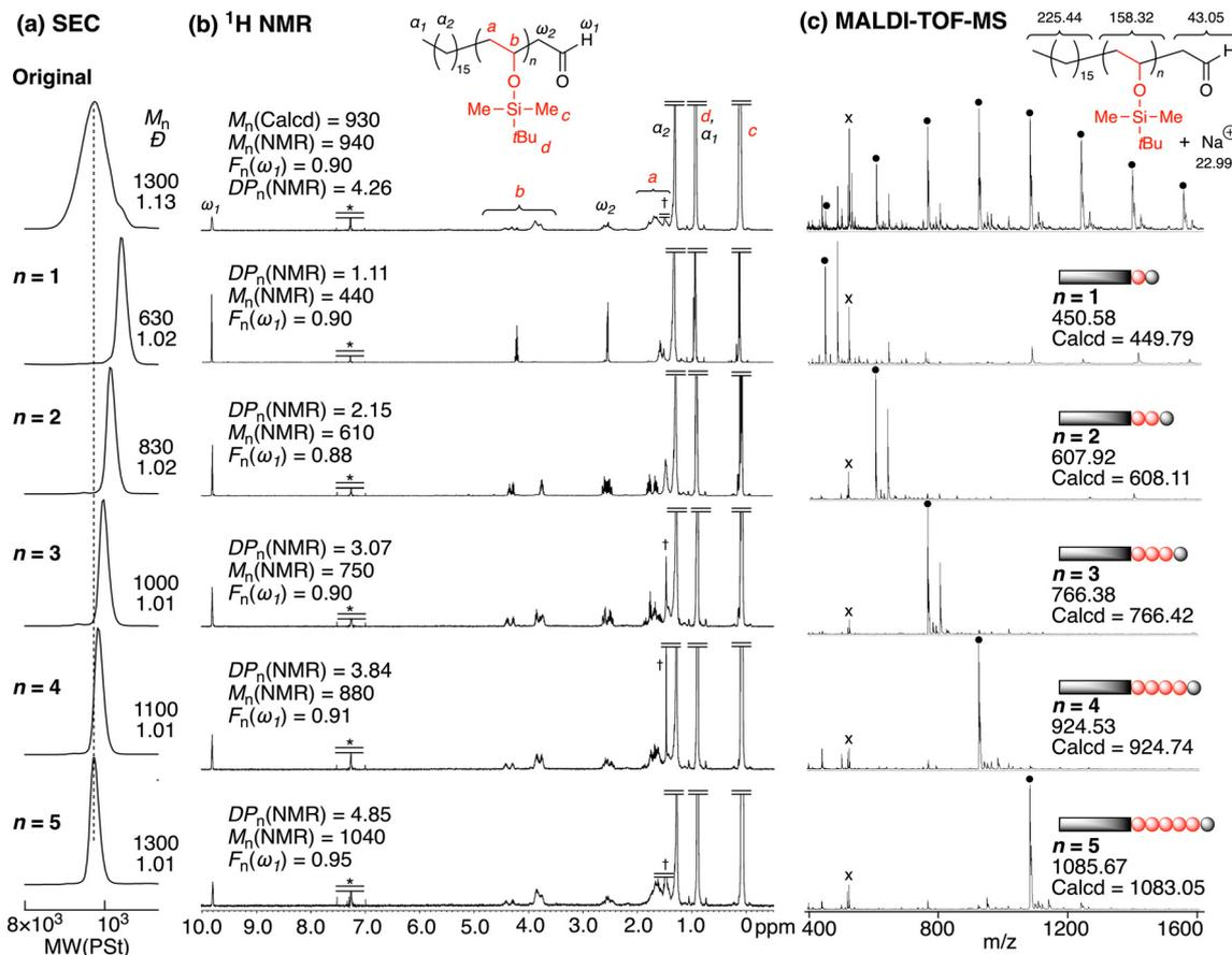
**Fig. 3** SEC (a), <sup>1</sup>H NMR (b), and MALDI-TOF-MS (c) spectra of monodisperse oligo(TBSVE) fractionated by preparative recycling SEC. \*CHCl<sub>3</sub> and <sup>†</sup>water in (b). The peaks marked with "x" in (c) are derived from *trans*-2-[3-(4-*tert*-butylphenyl)-2-methyl-2-propenyldene]malononitrile (DCTB) as the ionizing matrix.
