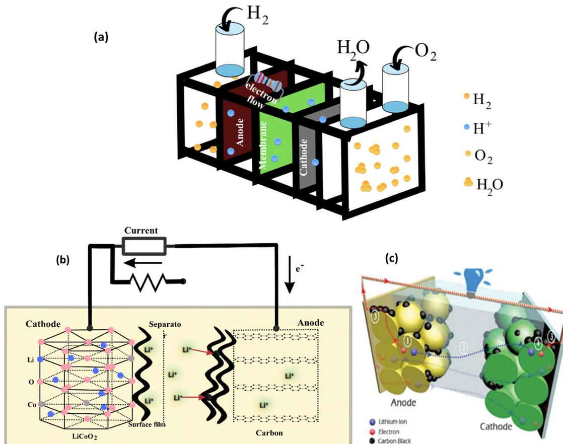
Fig. 17 (a) Diagram of a basic fuel cell. (b) Schematic of a typical lithium-ion battery featuring a graphite anode and a  $LiCoO_2$  cathode. (c) Illustration of lithium-ion and electron transport routes during the battery discharge process. Reproduced from ref. 100 with permission from Royal Society of Chemistry, copyright 2019.
