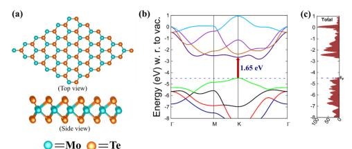
Fig. 2 (a) The top view and side view of the 2D monolayer MoTe<sub>2</sub> TMD; (b) electronic band structure and (c) total density of states (DOSs) of the 2D monolayer MoTe<sub>2</sub> TMD, obtained by the B3LYP-D3 DFT method.
