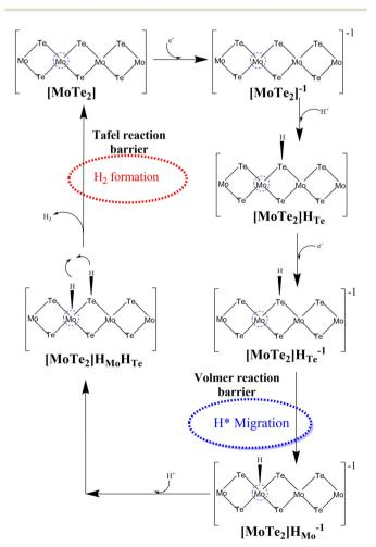
Fig. 6 Volmer-Tafel HER mechanism with the detailed two-electron transfer reaction pathway on the surface of the 2D MoTe $_2$  material.
