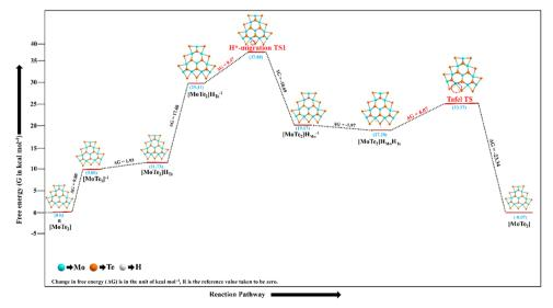
Fig. 8 The PES of the Volmer-Tafel reaction mechanism is shown here as it occurs during the HER process at the surface of the MoTe<sub>2</sub> material.
