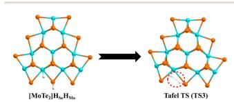
Fig. 7 The Volmer–Tafel reaction mechanism equilibrium geometries of  $[MoTe_2]H_{Mo}H_{Te}$  and TS3 are shown here.
