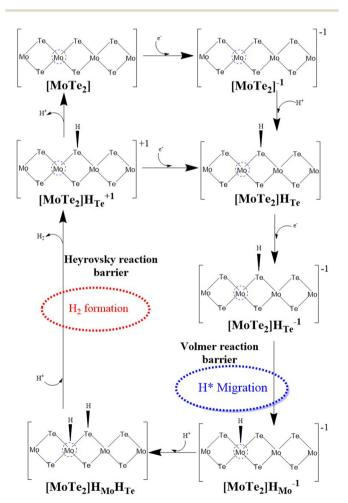
Fig. 3 Volmer-Heyrovsky HER mechanism of the detailed two electron transfer reaction pathways on the surface of the 2D MoTe<sub>2</sub> material.
