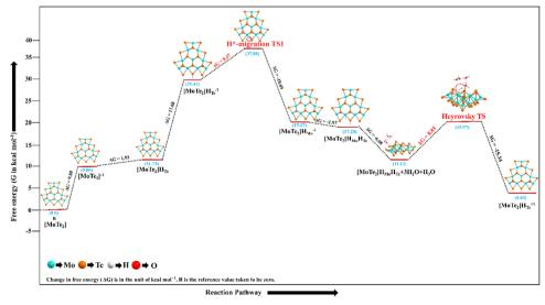
Fig. 5 The HER pathway followed by the Volmer-Heyrovsky reaction mechanism is shown here as it occurs during the HER process at the surface of the 2D monolayer MoTe<sub>2</sub> material
