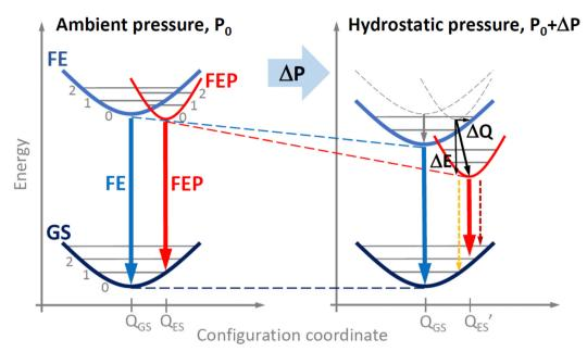
Fig. 5 Pressure induced changes in configuration diagram for free exciton and free exciton-polaron transition in EA<sub>2</sub>PbI<sub>4</sub>.
