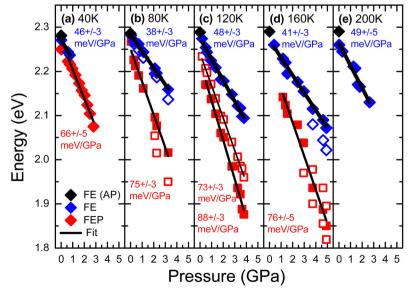
Fig. 4 Energies of the FE (blue solid squares) and the FE polaron (red solid squares) obtained from PL measurements of EA<sub>2</sub>PbI<sub>4</sub> at different hydrostatic pressure at (a) 40 K, (b) 80 K, (c) 120 K, (d) 160 K, and (e) 200 K. Black square - energies of FE at atmospheric pressure (AP); open squares - satellite peaks.
