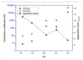
Fig. 7 Am-241 and Eu-152 sorption in binary competitive solution with an equimolar ratio by ZrPyTri2 (pH 1-3, contact time: 24 h). Vertical error bars represent counting errors that are too small to be visible on the scale of this figure.
