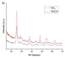
Fig. 5 Powder XRD patterns presented for a) bare zirconia and ZrPyTri2, and b) bare titania and TiPyTri.
