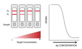
Fig. 1 Schematic representation of LFA signal outputs. (A) Sandwich format: an increase in target analyte concentration leads to a higher intensity of the test line (TL), resulting in a positive correlation between analyte concentration and signal intensity. (B) Competitive format: an increase in target analyte concentration results in a reduction of signal intensity on the TL, demonstrating an inverse correlation between analyte concentration and signal intensity.
