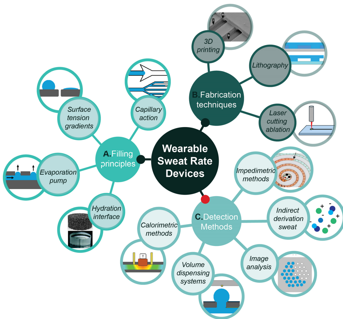
Fig. 1 Schematic overview of the A) filling principles, B) fabrication techniques and C) detection methods involved in the development of wearable microfluidic sweat rate devices. Reproduced with permission. 20–23 Hydration interface upper icon: Copyright 2024, Biomicrofluidics . Hydration interface lower icon: Copyright 2017, Lab Chip . 3D printing icon: Copyright 2017, Anal. Chem. Impedimetric methods: Copyright 2022, ACS Sens.
