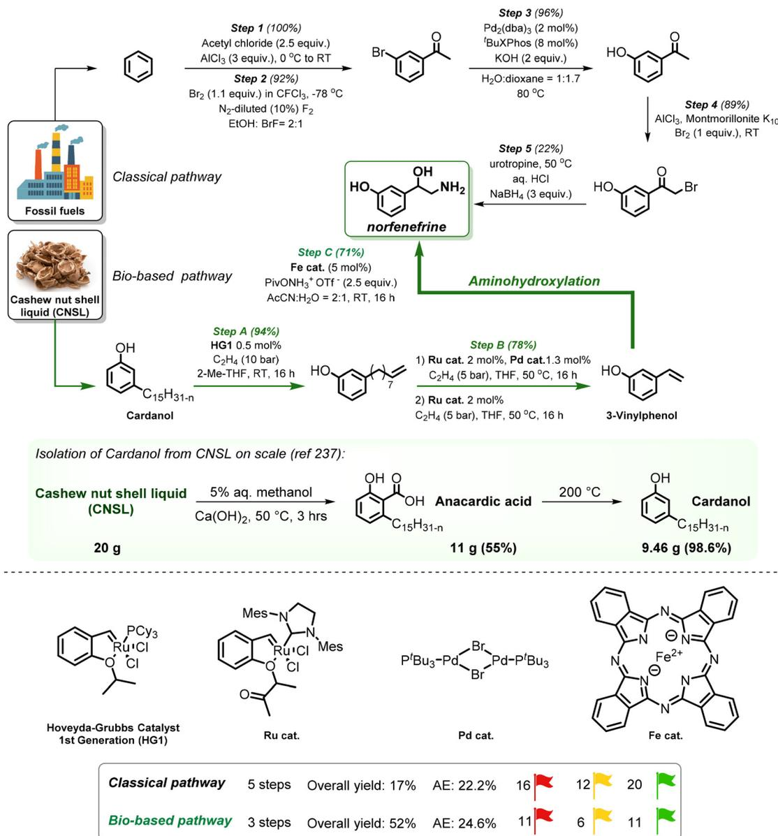
**Scheme 3** Synthesis of norfenefrine by the classical pathway (Steps 1–5) vs. the bio-based pathway (Steps A–C).
