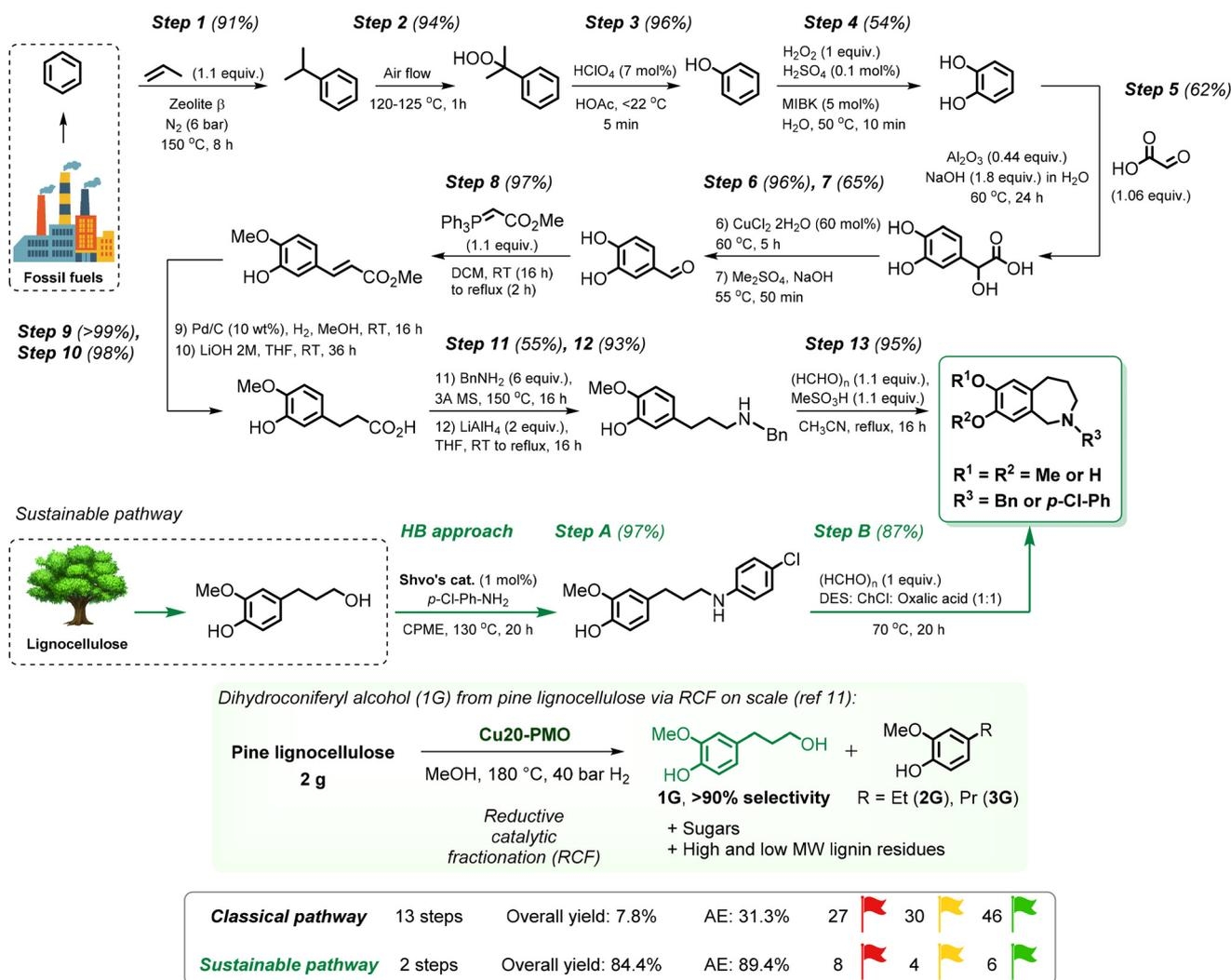
**Scheme 1** Synthesis of *N*-substituted tetrahydro-2-benzazepines via a classical route (Steps 1–13) starting from benzene vs. a sustainable route (Steps A–B) starting from lignin-derived dihydroconiferyl alcohol.
