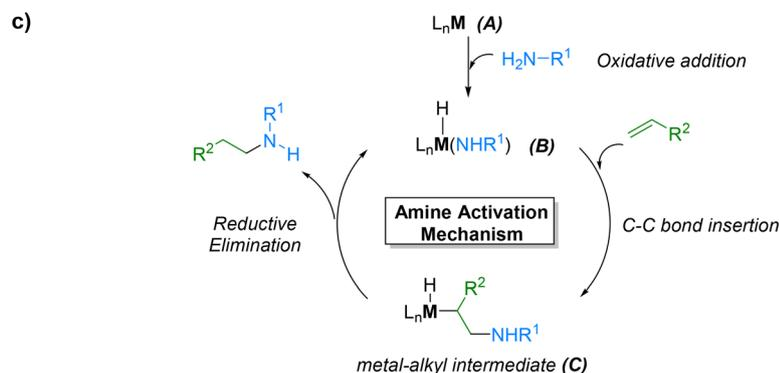
**Fig. 6** General scheme of the hydroamination of alkenes and overview of mechanisms: (a) the amido-mechanism typical of alkali and alkaline metals, lanthanides and actinides; (b) the C–C multiple bond mechanism and (c) the amine activation mechanism that are typical of late transition metals. All mechanisms shown lead to the anti-Markovnikov product. The same pathways apply to the Markovnikov product, but are not depicted due to space constraints.
