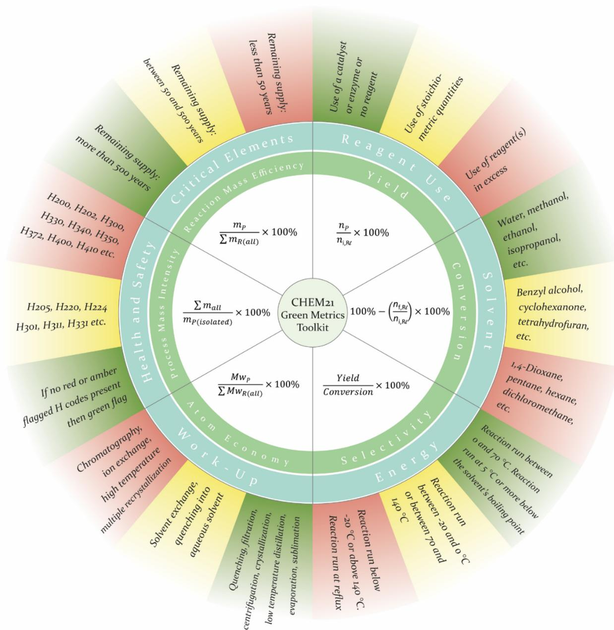
**Fig. 2** Overview of the first pass CHEM21 green metrics toolkit: quantitative (inner circle) and qualitative parameters (outer circle). Abbreviations:  $R$  – reactant;  $R_l$  – limiting reactant;  $P$  – product;  $n_p$  – moles of product formed;  $n_{i,R_l}$  – initial moles of limiting reactant;  $n_{f,R_l}$  – moles of limiting reactant left;  $m$  – mass;  $M_w$  – molecular weight.
