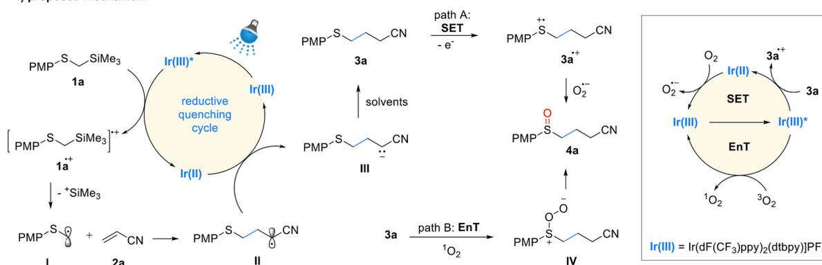
**Scheme 3** Controlled experiments and proposed mechanism. <sup>a</sup>Standard conditions: **1a** (0.2 mmol), **2a** (2.0 equiv.), Ir(dF(CF<sub>3</sub>)ppy)<sub>2</sub>(dtbpy)PF<sub>6</sub> (0.5 mol%), EtOH: pH = 9 buffer (5 : 1, 0.1 M), Ar, room temperature, 4 h. See ESI† for details.
