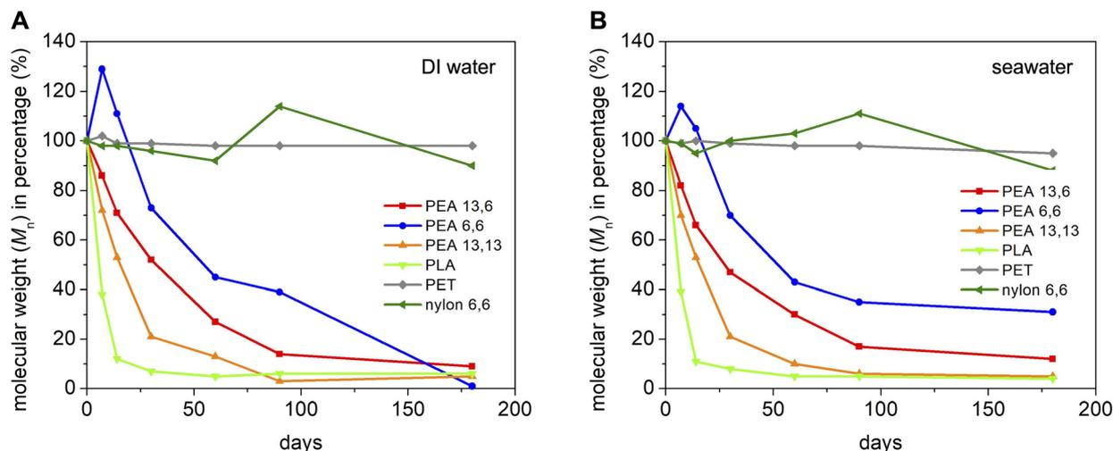
**Fig. 4** High-temperature hydrolytic degradation study of PEA 13,6, PEA 6,6, PEA 13,13, PLA, PET, and nylon 6,6 in DI water (A) or seawater (B). Vials were agitated in a water bath shaker held at 60 °C for specific durations: 1 week, 2 weeks, 1 month, 2 months, 3 months, and 6 months. The water-degradability was evaluated by the change in the number average molecular weight compared to the initial value.
