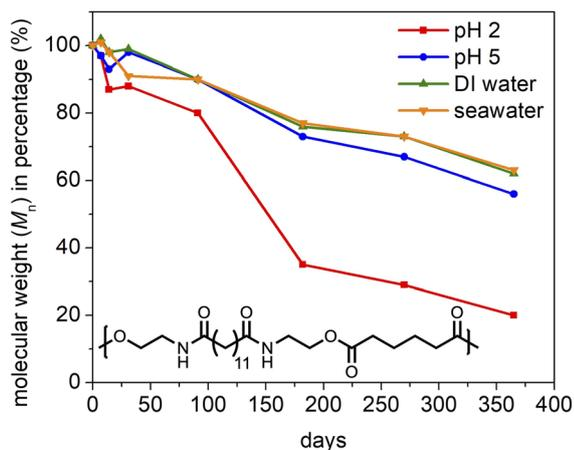
**Fig. 3** Hydrolytic degradation study of PEA 13,6 in four different aqueous media: pH 2, pH 5, DI water, and seawater. The samples were agitated on an orbital shaker at room temperature for specific durations (1 week, 2 weeks, 1 month, 3 months, 6 months, 9 months, and 12 months). The water-degradability was evaluated by the change in the number average molecular weight compared to the initial value.
