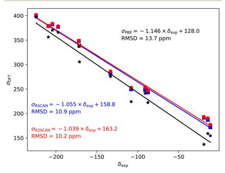
Fig. 2  $^{19}$ F magnetic shieldings,  $\sigma$ , calculated with the PBE (black), rSCAN (blue) and  $r^2$ SCAN (red) functionals vs. experimental chemical shifts,  $\delta$ . For each functional the line of best fit is given.
