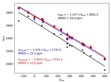
Fig. 5  $^{79/81}$ Br magnetic shieldings,  $\sigma$ , calculated with the PBE (black), rSCAN (blue) and r<sup>2</sup>SCAN (red) functionals vs. experimental chemical shifts,  $\delta$ . For each functional the line of best fit is given.
