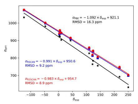
Fig. 4  $^{35/37}$ Cl magnetic shieldings,  $\sigma$ , calculated with the PBE (black), rSCAN (blue) and  $r^2$ SCAN (red) functionals vs. experimental chemical shifts,  $\delta$ . For each functional the line of best fit is given.
