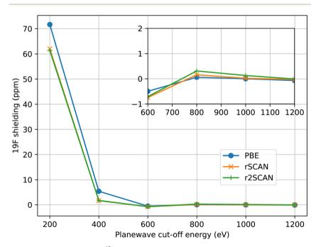
Fig. 1 Convergence of the  $^{19}$ F magnetic shielding in MgF $_2$  with size of the plane-wave basis. Shieldings are given relative to the value at 1600 eV. The inset figure shows the close-up of the range from 600–1200 eV.
