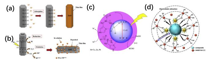
Fig. 6 Mechanisms of heavy metal ion removal using ZnO or TiO<sub>2</sub> particles via (a) adsorption on ZnO (ref. 83), (b) reduction/oxidation process on ZnO (ref. 83) and (c) photocatalysis on TiO<sub>2</sub> (ref. 82). d) Potential reactions involved in the adsorption of metal ions by magnetic iron oxide nanoparticles.84
