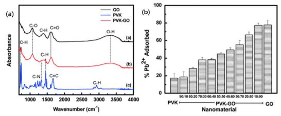
Fig. 10 a) ATR-IR spectra of graphene oxide (GO), poly(N-vinylcarbazole) (PVK), and PVK-GO polymer nanocomposite. b) Lead (Pb<sup>2+</sup>) adsorption at varying PVK-GO concentration ratios. 119
