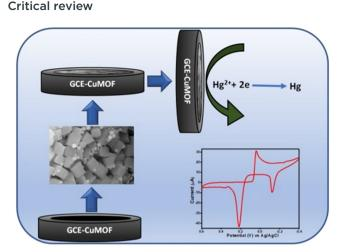
Fig. 16 Schematic diagram of copper metal organic framework nanoparticles for electrochemical detection of mercury (Hg<sup>2+</sup>). 170
