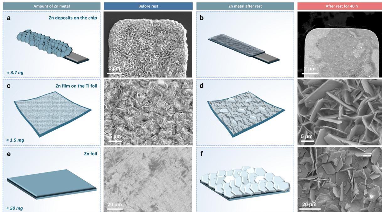
Fig. 4 Schematic illustrations and SEM images of electrodes with increasing quantity of Zn metal before and after resting in a 1 M  $\text{ZnSO}_4$  electrolyte vial for 40 hours. (a) and (b) Zn deposited to  $1 \text{ mA h cm}^{-2}$  on a liquid cell TEM chip Pt electrode (approximately 3.7 ng of Zn). (c) and (d) A thin Zn film deposited on a Ti foil electrode (approximately 1.5 mg of Zn). (e) and (f) Zn foil electrode (approximately 50 mg of Zn).
