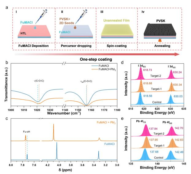
Fig. 1 (a) Process diagram of the one-step spin-coating method for preparing target perovskite films. (b) FTIR spectra of FuMACl and FuMACl/Pbl<sub>2</sub> complex. (c) Chemical shift information of FuMACl and FuMACl/Pbl<sub>2</sub> complex obtained from <sup>1</sup>H NMR measurements. (d) and (e) XPS spectra of the control, target-1 and target-2 perovskite films.
