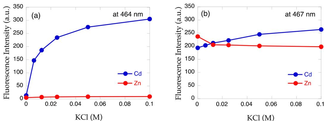
Fig. 9 Fluorescence intensity plot of (a) **14** and (b) **15** in the presence of  $\text{Cd}^{2+}$  (blue) or  $\text{Zn}^{2+}$  (red) with increasing amount of KCl. Adapted from ref. 30 with permission from American Chemical Society, copyright 2024.
