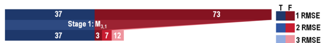
Fig. 6 A one-stage screening workflow for materials with a triplet excitation energy in the infrared, below 1.6 eV, based on the M_{3,1} model. The number of true positives (shades of blue) and the number of false positives (shades of red/pink) that pass the screening is shown when the thresholds are set to one, two, and three times the training set RMSE of the model.
