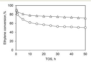
Fig. 10 Ethylene conversion vs. time on stream in the presence of (0)  $C_2H_4 + N_2$  and ( $\Delta$ )  $C_2H_4 + N_2 + H_2$  over the Ni-ASA catalyst. Reaction conditions: T = 250 °C, P = 1.5 MPa, WHSV = 1.1 h<sup>-1</sup>. This scheme has been reproduced from ref. 39.
