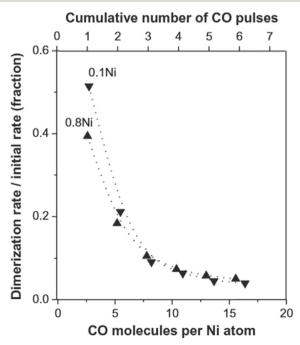
Fig. 6 Ratio of rates after each CO pulse introduction (per Ni) at -30 °C, 1.5 MPa ethene. This figure has been reproduced from ref. 52 with permission from Elsevier, copyright 2025.
