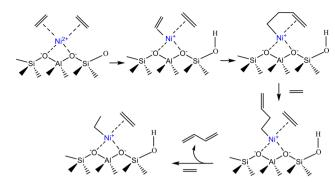
Scheme 7 Formation of the active center over the Ni-Beta catalyst. This scheme has been adapted from ref. 13 with permission from Elsevier, copyright 2025.
