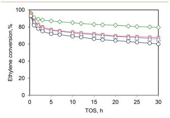
Fig. 7 Ethylene conversion vs. time on stream for various feed compositions ( $\square$ ) C<sub>2</sub>H<sub>4</sub> + N<sub>2</sub>, ( $\lozenge$ ) C<sub>2</sub>H<sub>4</sub> + N<sub>2</sub> + H<sub>2</sub> and ( $\triangle$ ) C<sub>2</sub>H<sub>4</sub> + N<sub>2</sub> + CO and ( $\circ$ ) C<sub>2</sub>H<sub>4</sub> + N<sub>2</sub> + H<sub>2</sub>O, over Ni-AlSBA-15 catalyst. Reaction conditions: T = 250 °C, P = 15 bar, WHSV = 1.1 h<sup>-1</sup>. This scheme has been reproduced from ref. 39.
