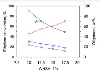
Fig. 5 Ethylene conversion and oligomer distribution at various WHSV; Ni-SBA-15 catalyst; ( $\lozenge$ ) % ethylene conversion, ( $\square$ ) % C<sub>4</sub>, ( $\Delta$ ) % C6, (x)  $C_{8+}$ ; conditions: 3.0 MPa of ethylene,  $T = 150 \, ^{\circ}$ C, TOS = 1 h. This scheme has been reproduced from ref. 40.
