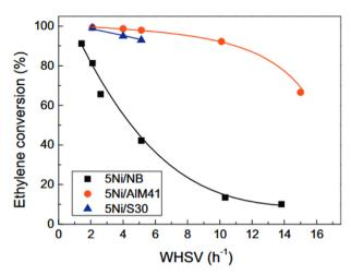
Fig. 9 Ethylene conversion over Ni-Beta (5Ni/NB), Ni-MCM-41 (5Ni/ AlM41) and Ni-ASA (5Ni/S30) catalysts. Reaction conditions: T = 120°C,  $P_{\text{tot}}$  = 3.5 MPa,  $P_{\text{C2}}$  = 2.6 MPa. This figure has been reproduced from ref. 12 with permission from Elsevier, copyright 2025.
