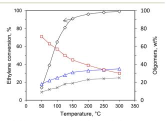
Fig. 4 Ethylene conversion and oligomer distribution at various temperatures; Ni-SBA-15 catalyst; (◊) % ethylene conversion, (□) % C4, ( $\Delta$ ) % C6, (x) C8; conditions: 3.0 MPa, WHSV = 10 h<sup>-1</sup>. This scheme has been reproduced from ref. 40.
