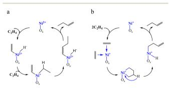
Scheme 2 Simplified Cossee–Arlman (a) and metallacycle mechanisms (b) ( $O_s$  = surface oxide ions).
