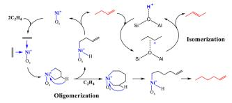
**Scheme 11** Proposed catalytic cycles for linear ethylene oligomerization involving Ni $^+$  and H $^+$  as active sites on the Ni-AlSBA-15 catalyst ( $O_s^{2-}$  = surface oxide ions). This scheme has been adapted from ref. 40.
