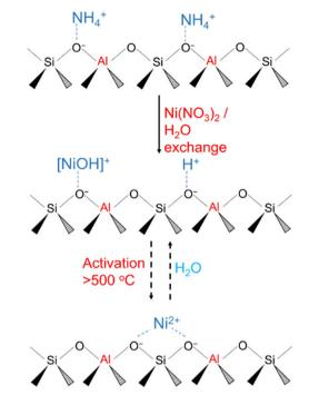
Fig. 1 General protocol for preparing the Ni-Beta catalyst. This figure has been adapted from ref. 14.
