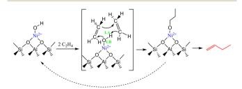
Scheme 12 Probable ethene dimerization catalytic cycle on (Ni-OH)<sup>+</sup> moieties acting as a Lewis acid-base pair proposed from a DFT analysis of ethene reactions on Ni-Al-MCM-41. This scheme has been adapted from ref. 51 with permission from American Chemical Society, copyright 2025.
