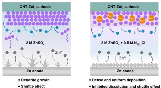
**Triethyl methyl ammonium ionic liquid as an effective electrolyte additive for high-performance zinc–iodine batteries**
