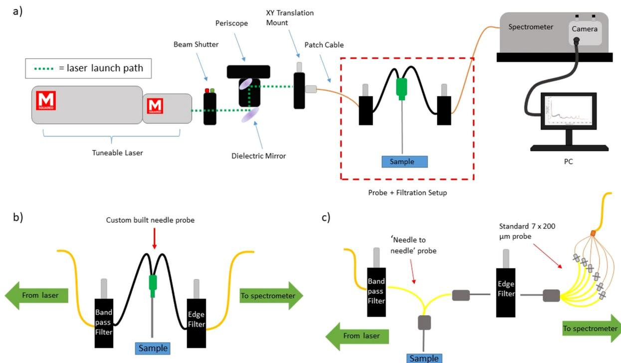
**Fig. 2** (a) A schematic of the overall SERDS setup of the experiment, with a red inset box identifying the 'probe + filtration' part of the setup. (b) Option 1 for the 'probe + filtration' configuration (Raman needle probe #1), used within all animal tissue measurements. (c) Option 2 for the 'probe + filtration' configuration (Raman needle probe #2), used within the lymph node measurements.
