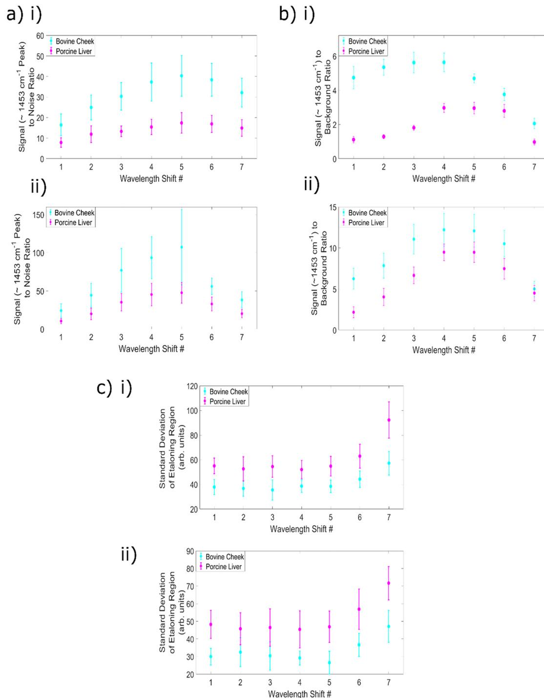
**Fig. 5** All calculated values as a function of wavelength shift number, with acquisition time = (40 s) and subplots (i) representing the SERDS difference spectra, subplots (ii) the reconstructed SERDS spectra. (a) Signal (1453 cm<sup>-1</sup>) to noise ratio. (b) Signal (1453 cm<sup>-1</sup>) to background ratio. (c) Mean standard deviation of etaloning region.
