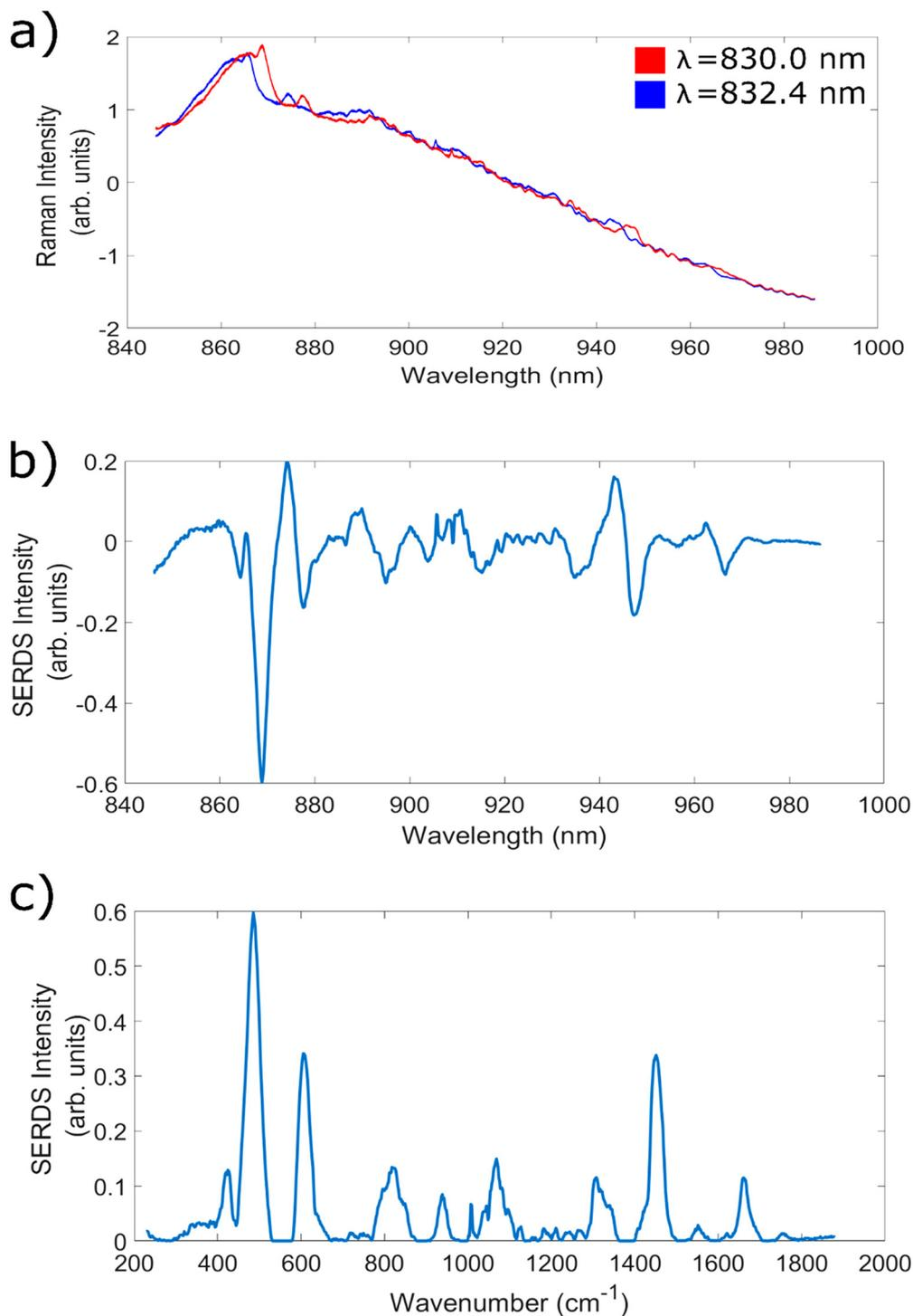
**Fig. 4** (a) Average bovine cheek spectra taken with 830.0 nm and 832.4 nm excitation and needle probe #1. Acquisition time =  $15 \times 20$  s. (b) Corresponding average SERDS difference spectra, acquisition time =  $15 \times 40$  s. (c) Corresponding average SERDS reconstruction.
