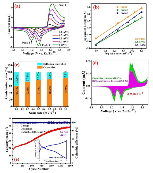
Fig. 4 (a) CV curves of  $Mn_3O_4$  nanoparticles cathode at different scan rates, (b)  $\log i$  and  $\log v$  plots resulted from Fig. 4a, (c) the capacitive/diffusion contribution ratios in  $Mn_3O_4$  nanoparticles cathode electrode, (d) capacitive contribution to the total capacity at a scan rate of 0.1 mV s<sup>-1</sup>, and (e) cycling performance operated at -10 °C at 0.2 A g<sup>-1</sup> and inset is discharge/charge profiles of the cycle number 1500.
