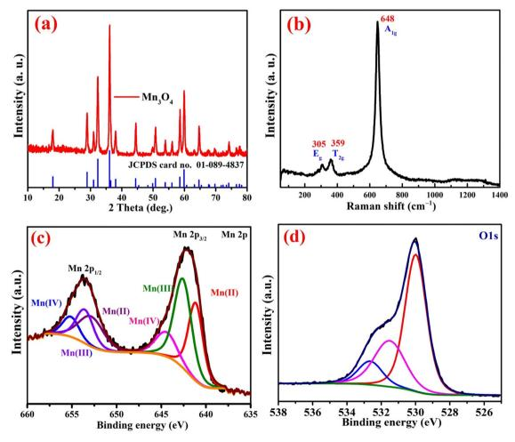
Fig. 1 (a) XRD pattern, (b) Raman spectrum, (c) Mn 2p XPS high-resolution spectrum, and (d) O 1s XPS high-resolution spectrum of the produced  $Mn_3O_4$  nanoparticles.
