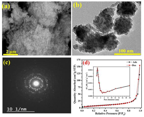
Fig. 2 (a) SEM image, (b) TEM Image, (c) SAED, and (d) Nitrogen adsorption and desorption isotherm (inset shows the pore distribution) of the produced Mn<sub>2</sub>O<sub>4</sub> nanoparticles
