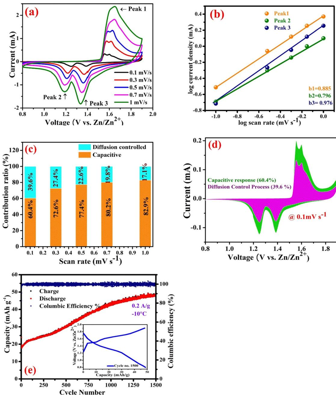
Fig. 4 (a) CV curves of Mn<sub>3</sub>O<sub>4</sub> nanoparticles cathode at different scan rates, (b) log *i* and log *v* plots resulted from Fig. 4a, (c) the capacitive/diffusion contribution ratios in Mn<sub>3</sub>O<sub>4</sub> nanoparticles cathode electrode, (d) capacitive contribution to the total capacity at a scan rate of 0.1 mV s<sup>-1</sup>, and (e) cycling performance operated at -10 °C at 0.2 A g<sup>-1</sup> and inset is discharge/charge profiles of the cycle number 1500.
