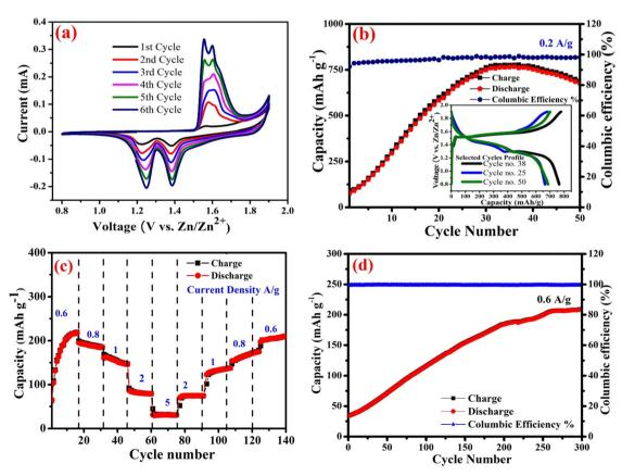
Fig. 3 Electrochemical performances of the  $Mn_3O_4$  nanoparticles cathode: (a) CV curves at a scan rate of 0.1 mV s<sup>-1</sup>, (b) cycle performance at 0.2 A g<sup>-1</sup> and inset is discharge/charge profiles of selected cycles, (c) rate property, and (d) cycling performance at 0.6 A g<sup>-1</sup>.
