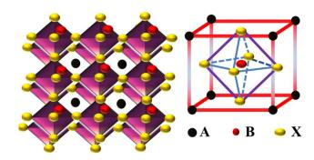
Fig. 1 Schematic diagram of the crystal structure of PSCs.<sup>32</sup>
