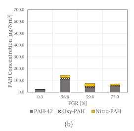
Fig. 1 Graphs showing the total PAH-42, oxy- and nitro-PAH concentrations in the off-gas at varying FGR levels for experiments at (a)  $1000 \text{ Nm}^3$  h<sup>-1</sup> and (b)  $500 \text{ Nm}^3$  h<sup>-1</sup>.
