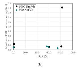
Fig. 6 Graphs showing the estimated PAH stack emissions for PAH-42 and substituted PAHs (sum of oxy- and nitro-PAHs) for both 1000  $\rm Nm^3$   $\rm h^{-1}$  and 500  $\rm Nm^3$   $\rm h^{-1}$  at varying FGR levels. (a) PAH-42 and (b) substituted PAH.
