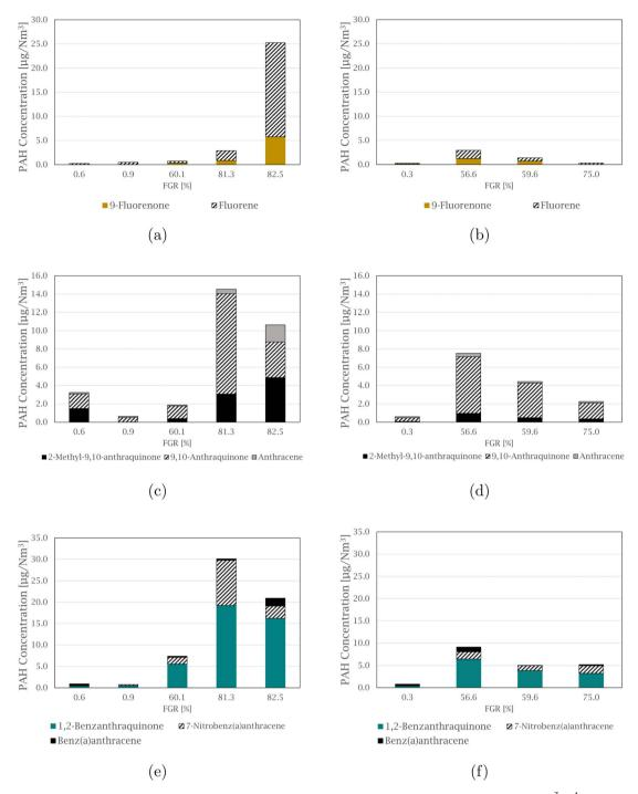
$\textbf{Fig. 5} \quad \textbf{Graphs showing the distribution of oxy-PAHs and the corresponding parent PAHs for experiments at 1000 \, \text{Nm}^3 \, \text{h}^{-1} \, \text{(left) and 500 Nm}^3 \, \text{h}^{-1} \, \text{(left)} \, \text{and 500 Nm}^3 \, \text{h}^{-1} \, \text{(left)} \,$ (right), (a and b): fluorene species, (c and d): anthracene species, and (e and f): benz(a)anthracene species.
