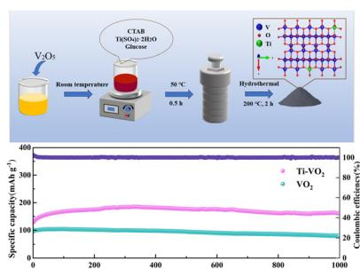
**Enhancing the stability of zinc-ion batteries with titanium-doped VO<sub>2</sub> cathode materials**
