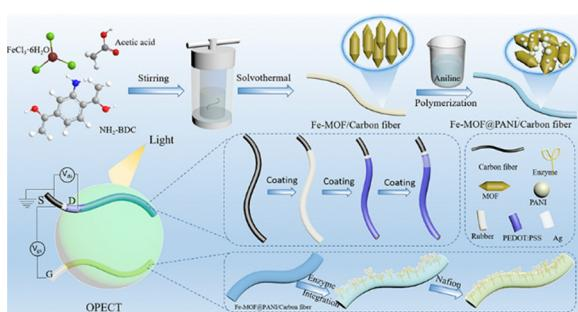
**An organic photoelectrochemical transistor based on the Fe-MOF@PANI/carbon fiber for uric acid detection**
