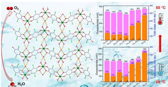
**CoNi-bimetallic coordination polymers as catalyst for boosting oxygen evolution reaction activity**
