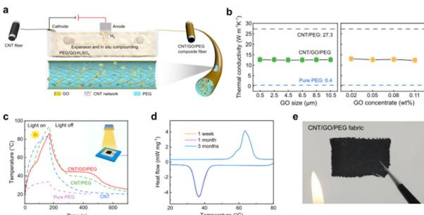
**Carbon nanotube graphene multilevel network based phase change fibers and their energy storage properties**
