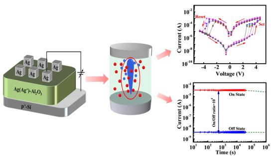
**Fabrication of a high performance memristor device by metallization of Ag<sup>+</sup> inside a solution processed Li<sub>5</sub>AlO<sub>4</sub> thin film**
