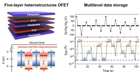
**High-performance multilevel nonvolatile organic field-effect transistor memory based on multilayer organic semiconductor heterostructures**
