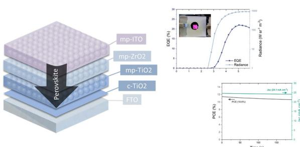
**Mesoscopic fully printable perovskite light-emitting diodes in the near infra-red region**
