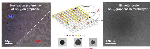
**Nucleation preference and lateral growth of monolayer tin disulfide on graphene**
