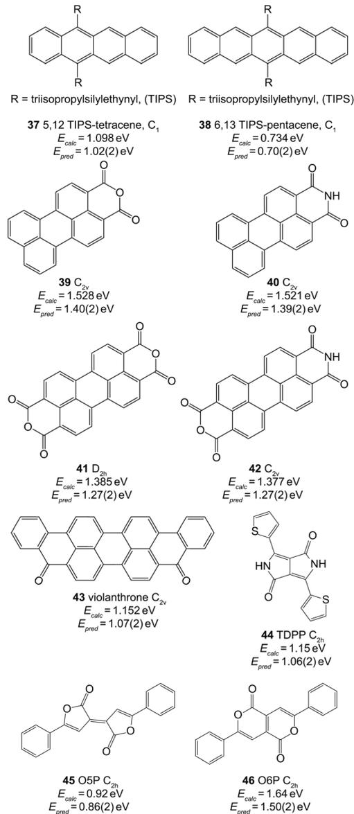
Fig. 4 Extended  $\pi$  systems and predicted values of  $E_{T_1}$  using B3LYP/3-21G and the parameters in the final row of Table 2. The symmetries used for the calculations are given next to each molecule.
