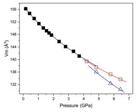
Fig. 7 Variation in unit-cell volume per formula unit  $(V_m)$  with pressure of CsCaCl<sub>3</sub>. The filled square for the cubic phase, unfilled red squares the tetragonal phase and the unfilled blue triangles the rhombohedral phase. The solid lines are the fitted Birch-Murnaghan EoS to the data points as described elsewhere. The number of formula units per unit cell (Z) of the cubic phase is 1, 4 for the tetragonal phase and 2 for the rhombohedral phase.
