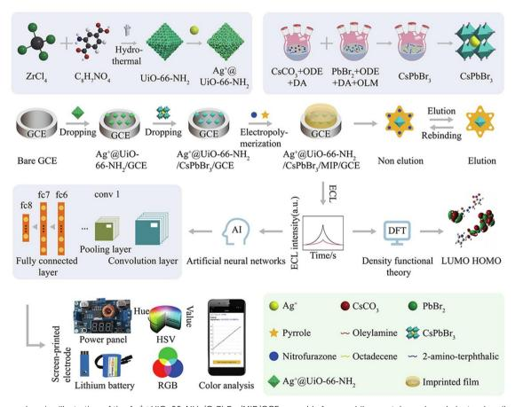
Fig. 4 A comprehensive illustration of the Ag+aUiO-66-NH<sub>2</sub>/CsPbBr<sub>3</sub>/MIP/GCE assembly for a mobile smartphone-based electrochemiluminescence molecularly imprinted polymer (ECL-MIP) system, depicting the intricate steps of preparation, integration of machine learning techniques, and the sensing mechanism. Adapted with permission. 123 Copyright 2022, Elsevier.
