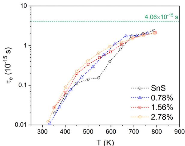
Fig. 5 Temperature-dependent electron relaxation time  $\tau_e$  for the pristine SnS and three Ag-doped SnS models obtained by fitting the measured  $S$  and  $\sigma$  to electrical-transport calculations. The value of  $\tau_e = 4.06 \times 10^{-15}$  s estimated from experimental data is shown by a horizontal dashed line for comparison.
