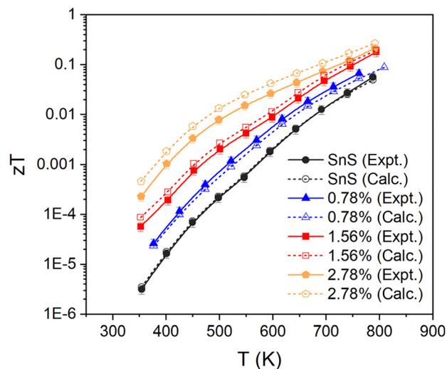
Fig. 8 Thermoelectric figure of merit  $zT$  of pristine and Ag-doped SnS ceramics. For each set of samples two sets of data are given: one obtained using the measured lattice thermal conductivity  $\kappa_L$  ("expt.", solid lines/solid symbols) and one using the calculated  $\kappa_L$  ("calc.", dashed lines/open symbols).
