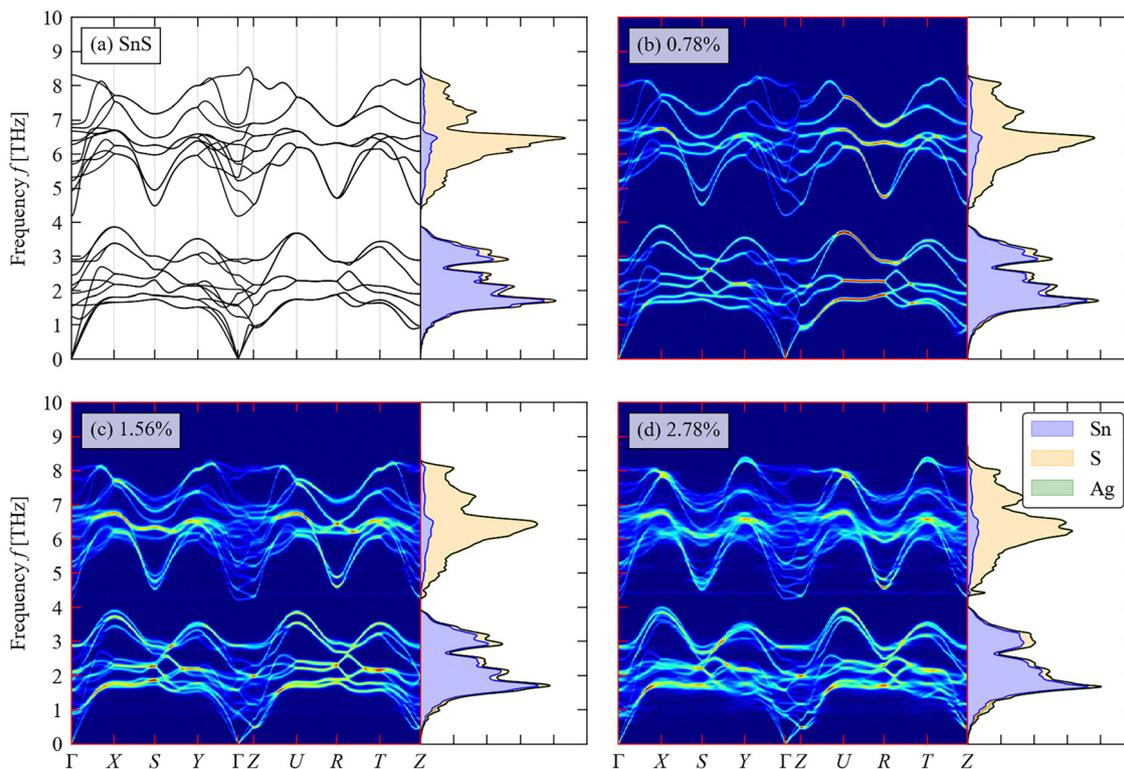
Fig. 6 Total and atom-projected phonon density of states (DoS) curves and calculated phonon dispersion along a high-symmetry path through the Brillouin zone (c.f. Fig. 3(c)) of pristine SnS (a) and (b)–(d) Ag-doped SnS with doping concentrations of 0.78 at% (b), 1.56 at% (c) and 2.78 at% (d).
