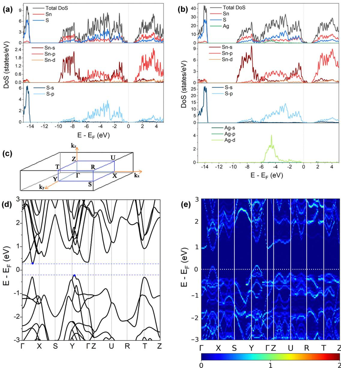
Fig. 3 (a) and (b) Total and atom-projected (partial) density of states of pristine SnS (a) and 2.78 at% Ag-doped SnS (b) calculated at the HSE06 level of theory. (c) *Pmcn* Brillouin zone with high-symmetry points marked. (d) and (e) Electronic band structures of pristine SnS (d) and 2.78 at% Ag-doped SnS (e) calculated at the PBEsol level of theory.
