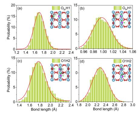
Fig. 3 Probability distributions of O<sub>br</sub>H bond lengths in (a) a single water molecule and (b) monolayer systems, and IHB lengths (c) after and (d) before water dissociation in the monolayer system.
