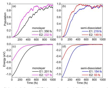
Fig. 5 (a and b) Dynamics of hole capture by the water HOMO in the monolayer and semi-dissociated systems, respectively. E1 and E2 represent high- and low-energy photogenerated hole donor states. (c and d) Energy relaxation processes in the monolayer and semi-dissociated systems, with E1 and E2 as the initial states.
