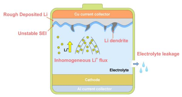
Fig. 15 Challenges of anode-free lithium metal batteries.
