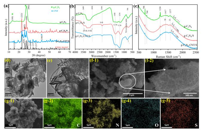
Fig. 1 For  $g-C_3N_4$ ,  $g-C_3N_4/S$ , and  $g-C_3N_4-CNT/S$ : (a) XRD patterns, (b) FTIR spectra and (c) Raman spectra; TEM images for (d)  $g-C_3N_4$  and (e)  $g-C_3N_4-CNT/S$  materials; (f) SEM images for  $g-C_3N_4-CNT/S$ ; (g) color mapping of  $g-C_3N_4-CNT/S$  demonstrating the uniform distribution of C, N, O, and S elements.
