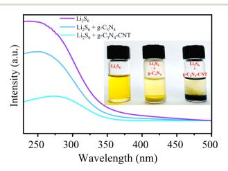
Fig. 3 UV-vis spectra for blank  $\rm Li_2S_6$  and  $\rm Li_2S_6$  added with CN and g-C<sub>3</sub>N<sub>4</sub>-CNT. The inset shows the digital picture of the effect of the active material on the adsorption of LiPSs in  $\rm Li_2S_6$  solution.
